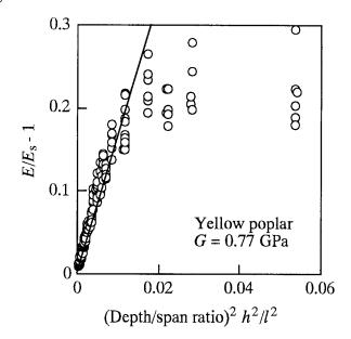
Fig. 2. Value of  $(E/E_s - 1)$  calculated by substituting the shear modulus obtained from the vibration tests into Timoshenko's bending theory corresponding to the squares of depth/span ratio
