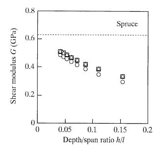
Fig. 3. Shear modulus corresponding to the depth/span ratio obtained from the finite element method (FEM) calculations when the grid point for measuring the deflection was varied. *Circles*, measured at the loading point; *squares*, measured at the middle of the depth; *triangles*, measured at the opposite side of the loading point; *broken line*, shear modulus given as a material parameter (G = 0.63 GPa for spruce)
