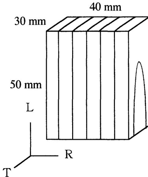
Fig. 1. Wood specimen for color measurement
