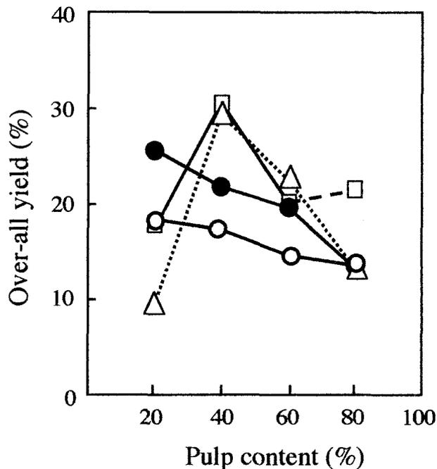
Fig. 6. Overall yield of AC sheets. Open circles, HAL; filled circles, SAL; triangles, KL; squares, WSL
