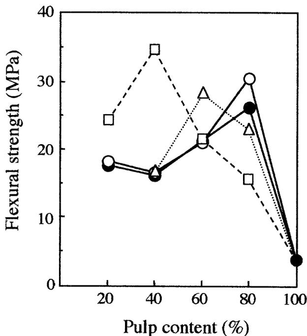
**Fig. 1.** Flexural strength of precursory sheets. *Open circles*, hardwood acetic acid lignans (HAL); *filled circles*, softwood acetic acid lignans (SAL); *triangles*, softwood kraft lignin (KL); *squares*, wheat-straw lignin (WSL)
