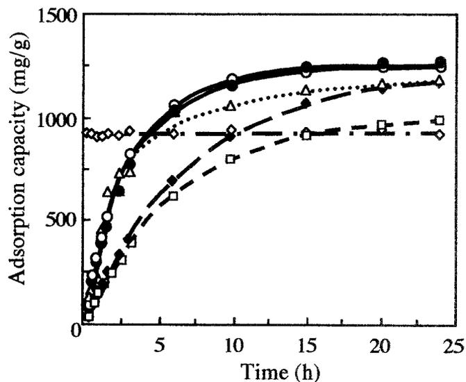
**Fig. 8.** Adsorption rate of *p*-chlorophenol onto activated carbon sheets. Open circles, HAL; filled circles, SAL; triangles, KL; squares, WSL
