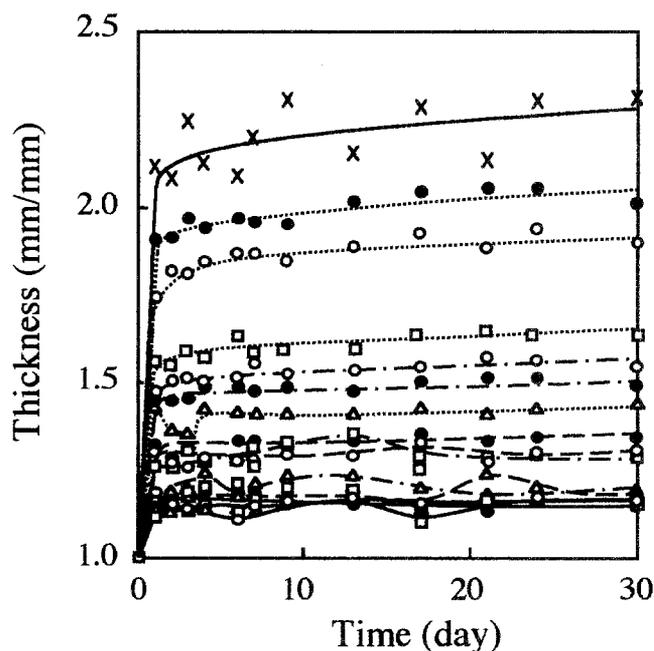
**Fig. 3.** Changes in thickness during 30 days of immersion in water. *Solid lines*, 20% pulp sheet; *broken lines*, 40% pulp sheet; *dashed lines*, 60% pulp sheet; *dotted lines*, 80% pulp sheet; *crosses*, 100% pulp sheet; *open circles*, HAL; *filled circles*, SAL; *triangles*, KL; *squares*, WSL
