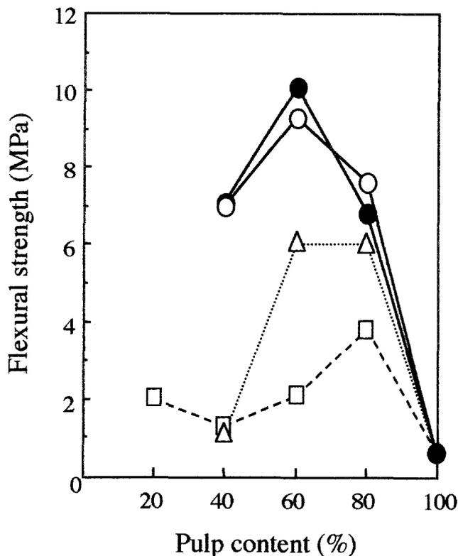
Fig. 5. Flexural strength of activated carbon sheets. Open circles, HAL; filled circles, SAL; triangles, KL; squares, WSL
