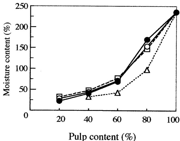
**Fig. 2.** Water absorptivity of precursory sheets after 30 days of immersion in water. *Open circles*, HAL; *filled circles*, SAL; *triangles*, KL; *squares*, WSL
