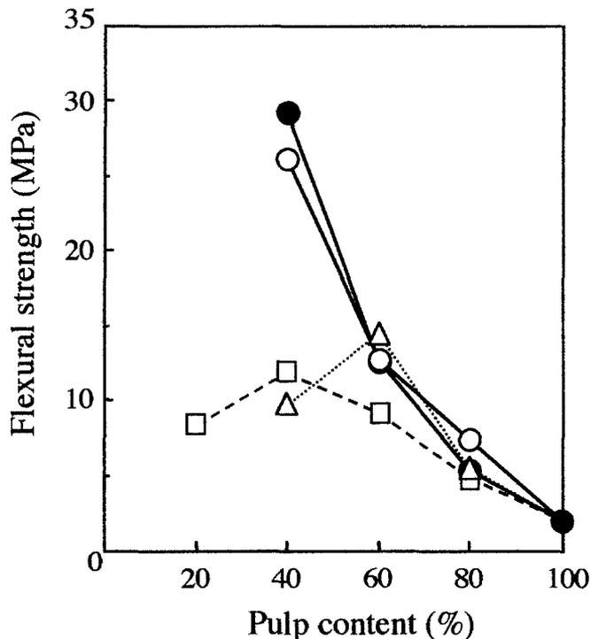
Fig. 4. Flexural strength of carbonized sheets. Open circles, HAL; filled circles, SAL; triangles, KL; squares, WSL
