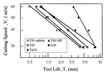
**Fig. 8.** Tool life and cutting speed relations for all tools investigated. Conditions: F 0.05mm/rev; D 1mm; WM, HDCB; tool life criterion 200 $\mu$ m
