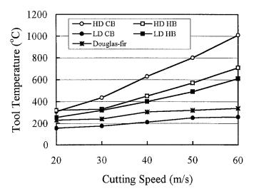
**Fig. 4.** Cutting tool temperatures as a function of the cutting speeds and work materials. HDCB, high-density wood-chip/cement board; *HDHB*, high-density hardboard; *LDCB*, low-density wood-chip/cement board; LDHB, low-density hardboard. Conditions: depth of cut (D) 0.05 mm; width of cut (W) 5 mm; cutting period 3 s. tools were K10 and cermet
