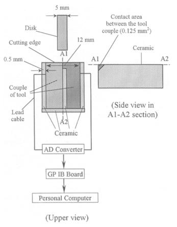
Fig. 3. Thermal electromotive force (EMF) measurement. *AD*, Aanalog to digital; *GP IB*, General purpose interface bus
