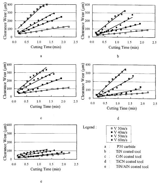
Fig. 6. Behaviors of the clearance wear of the tools tested with cutting speed at 1.3-min cutting time. Left Conditions: F 0.05 mm/rev; D 1 mm; T 1.3 min; WM, HDCB. Right Conditions: D 0.05 mm; W 5 mm; cutting period 3s; WM, HDCB. Tools were K10 and cermet
