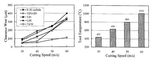
more, the hardness decreased at 800°C. The hardness of the TiCN coating was reported to be about 1100 HV at 800°C.<sup>6</sup> These data suggest that the wear rate and clearance wear of the TiCN-coated carbide tool were accelerated by oxidation of its coating film and the decreased hardness due to the high temperature.
