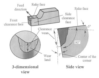
Fig. 2. Clearance wear measurement
