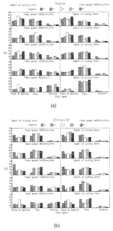
in conjunction with either the feed speed or the cutting depth was studied. The chip types could be distinguished into four groups – flake type, splinter type, flow type, granule type – according to chip sizes and shapes, respectively.
