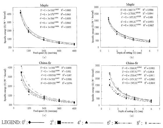
Fig. 6. Relations between feed speed, cutting depth, and specific energy while milling maple and China fir. *Diamonds*,  $0^\circ$ ; squares,  $2^\circ$ ; triangles,  $4^\circ$ ; ×,  $6^\circ$ ; \*,  $8^\circ$
