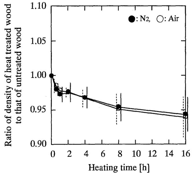
**Fig. 7.** Changes in density caused by heat treatment. The same specimens were used before and after treatment. *Filled circles*, specimens heat treated in  $N_2$  gas; *open circles*, specimens heat treated in air. *Solid lines at the right side of the filled circles and dashed lines at the left side of the open circles* are the standard deviation
