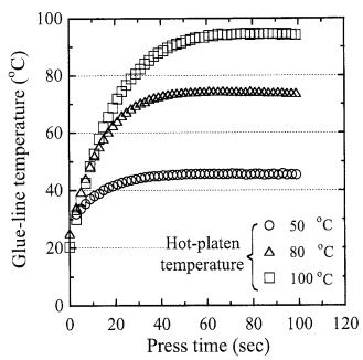
Fig. 11. Variation of glue-line temperature in three-ply plywood during hot-platen pressing. DF-1000/D-33 ratio is 25:75
