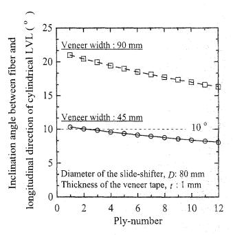
**Fig. 6.** Relations between ply number and calculated fiber inclination angle to the longitudinal direction of cylindrical LVL
