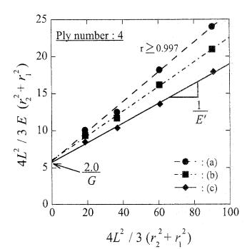
**Fig. 12.** Estimation of Young's modulus (E') and modulus of rigidity (G). (a) Veneer width 45 mm, press time 21 s. (b) Veneer width 45 mm, press time 42 s. (c) Veneer width 90 mm, press time 42 s. Productivity in (a) and (c) are equal, but in (b) it is half
