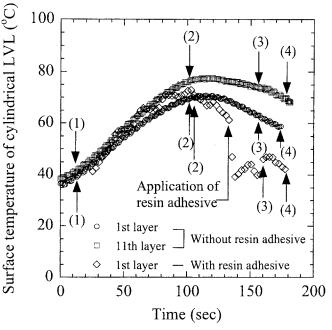
**Fig. 4.** Relations between time and surface temperature of cylindrical LVL. (1), (2), (3), (4) represent the initiation of heating, end of heating, initiation of pressing, and end of pressing, respectively, at a winding speed of 18.8 rad/min
