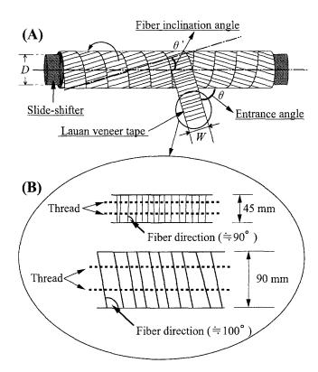
Fig. 5. Cylindrical LVL manufacturing process (A) and an enlargement of the sewn lauan veneer tape (B)
