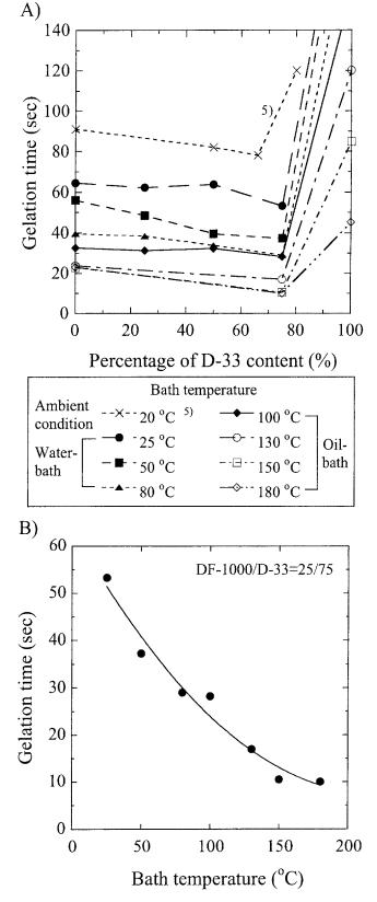
**Fig. 8.** A Effects of resin mix ratio and bath temperature on gelation time. The number "5" is a reference number. **B** Relations between gelation time and bath temperature at DF-1000/D-33 25:75
