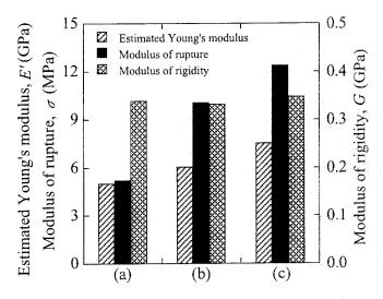
**Fig. 13.** Comparison of bending performance of cylindrical LVL (fourply) manufactured by various combinations of veneer width and press time. Refer to Fig. 12 for an explanation of (a), (b), and (c)
