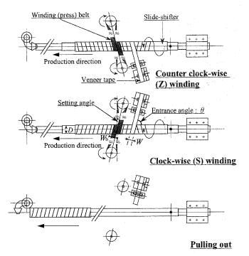
Fig. 1. Parts of the spiral-winder
