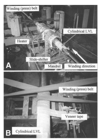
Fig. 3. Manufacturing process of cylindrical laminated veneer lumber (LVL). A Appearance of spiral-winder and pilot installed cylindrical heater. B Close-up view
