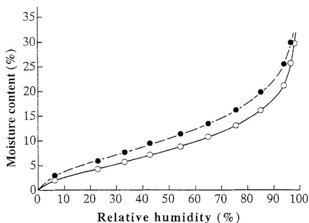
Fig. 1. Adsorption (open symbols) and desorption (solid symbols) isotherms of wood moisture-conditioned for a period of 50 weeks
