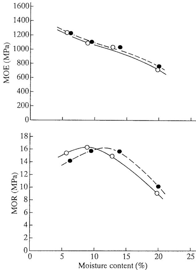
**Fig. 8.** Difference in MOE and MOR for wood moisture-conditioned for 4 weeks by the adsorption process (*open symbols*) and by the desorption process from a moisture content below the FSP (*solid symbols*) as a function of the moisture content
