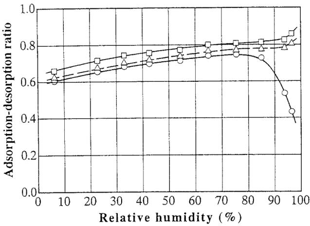
Fig. 2. Adsorption-desorption ratios for wood moisture-conditioned for 3 weeks (circles), 10 weeks (triangles), and 50 weeks (squares)
