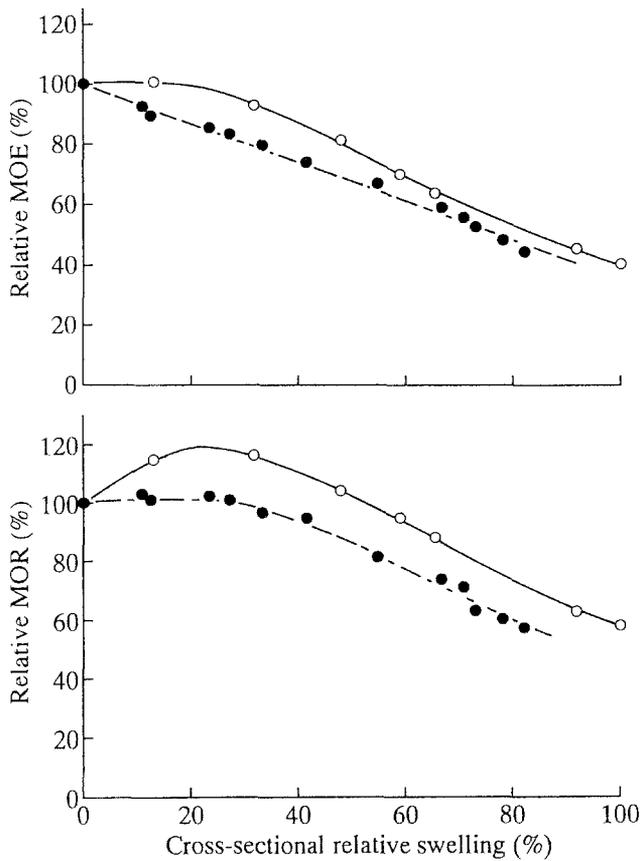
**Fig. 6.** Difference in modulus of elasticity (*MOE*) and modulus of rupture (*MOR*) for wood moisture-conditioned for 4 weeks by the adsorption process (*open symbols*) and by the desorption process from a water-saturated state (*solid symbols*) as a function of the cross-sectional relative swelling
