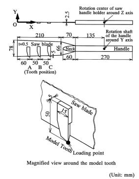
Fig. 2. Saw blade with model tooth
