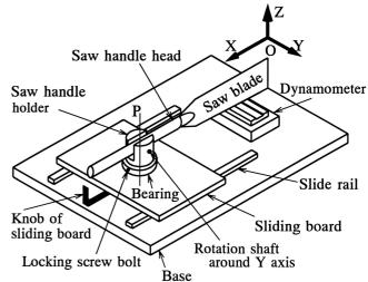
Fig. 3. Experimental device
