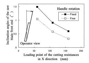
Fig. 10. Inclination of the saw blade by FEM calculation
