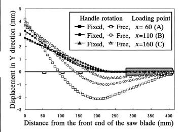
Fig. 9. Displacement of the top end of the saw by FEM calculation
