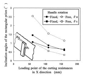
Fig. 11. Inclination of the rectangular prism by FEM calculation
