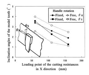
Fig. 7. Experimental inclination of the the model tooth.  $\theta_{\rm H}$ , inclination angle of model tooth from X direction in top view;  $\theta_{\rm S}$ , inclination angle of model tooth from a normal line in operator view
