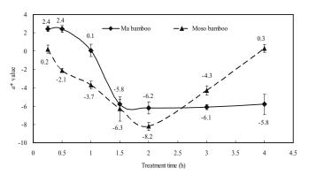
**Fig. 2.** Changes in *a*\* value for ma bamboo and moso bamboo culms after treatment with 0.25% ammoniacal copper quaternary compound-type B (ACQ-B) at 100°C for different times
