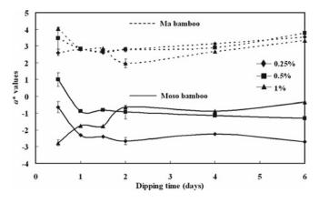
Fig. 3. Changes in  $a^*$  value of ma bamboo and moso bamboo treated with 0.25%, 0.5%, and 1% ACQ-B solution under ambient conditions for 6 days
