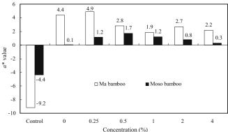
**Fig. 4.** Changes in *a*\* value of ma bamboo and moso bamboo treated with different concentrations of ACQ-B solution for 2 h using ultrasonic treatment
