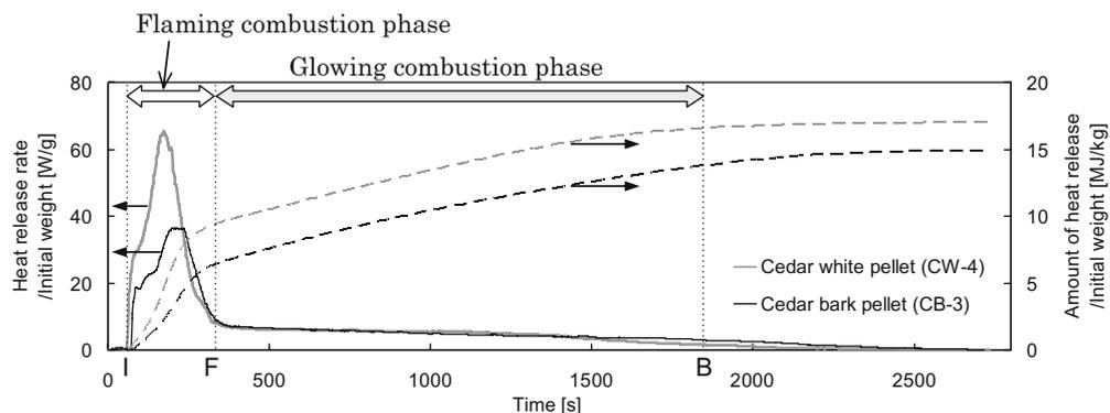
**Table 2.** Results of combustion test by cone calorimetry
