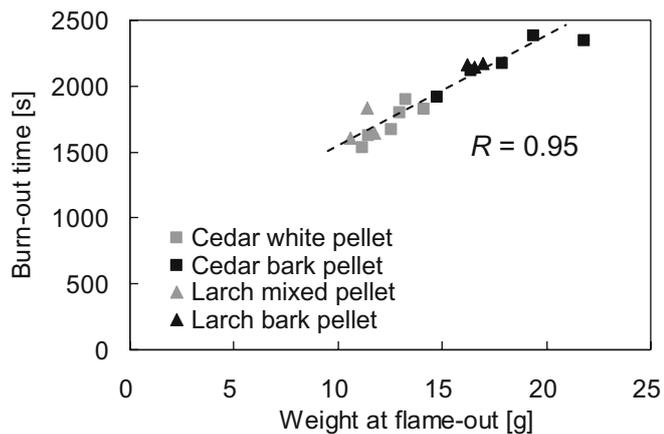
**Fig. 5.** Relationship between burn-out time and weight at flame-out point
