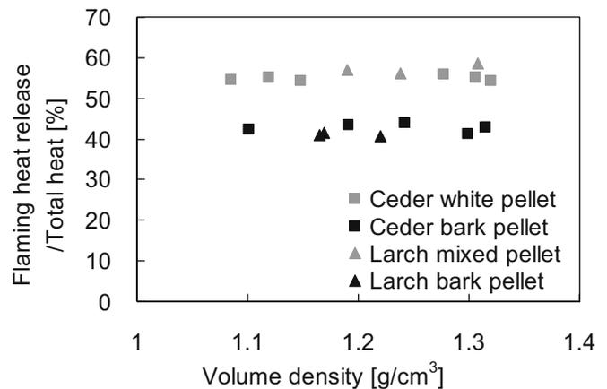
**Fig. 4.** Ratio of amount of heat release during flaming combustion to total heat release
