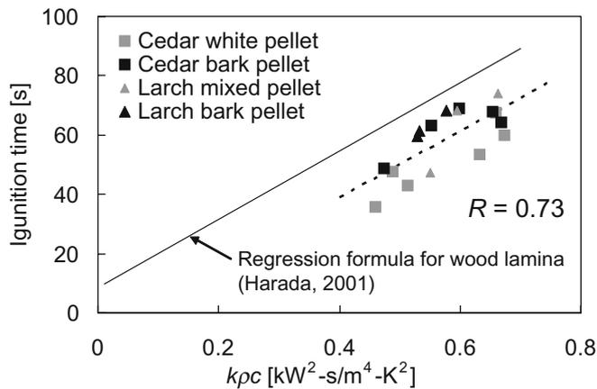
**Fig. 3.** Relationship between ignition time and heat inertia for four types of pellets
