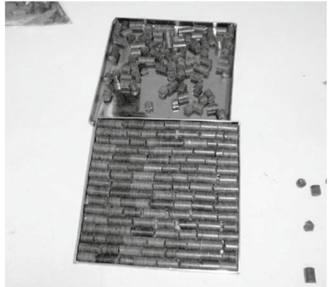
**Fig. 1.** Picture of the sample pan of the cone calorimeter
