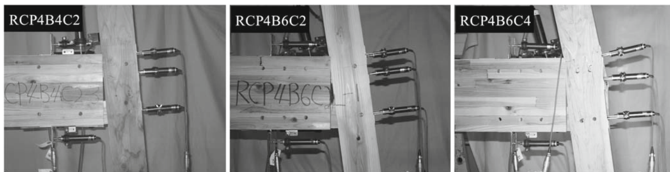
Fig. 11. Final stage of each type of joint on the rotational test
