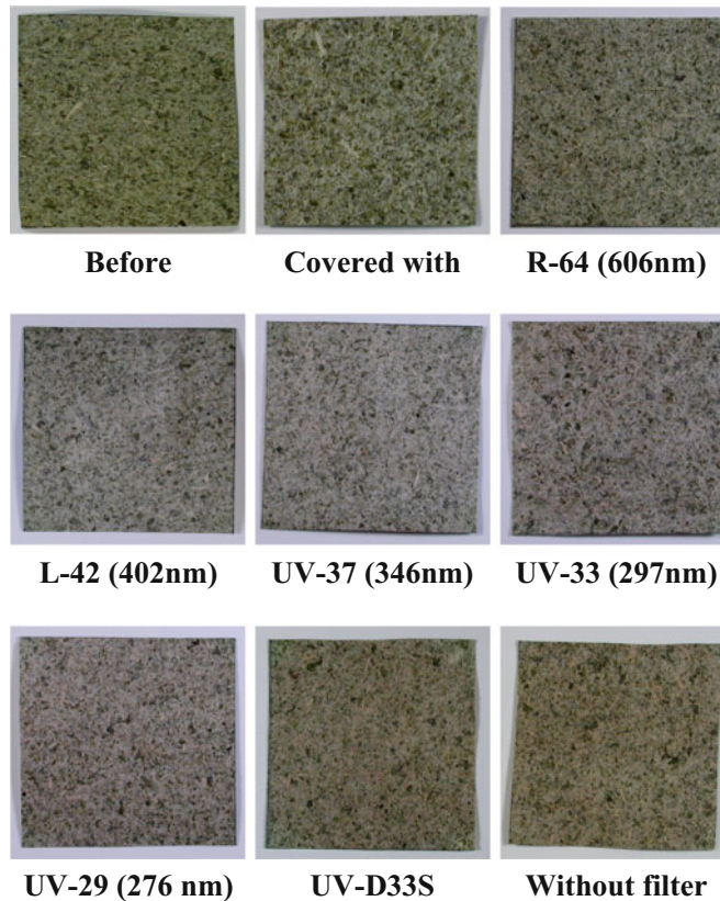
Fig. 8. Change in the color of papers containing 60 wt% of wasted green tea leaves on light irradiation for 1 h through different filters
