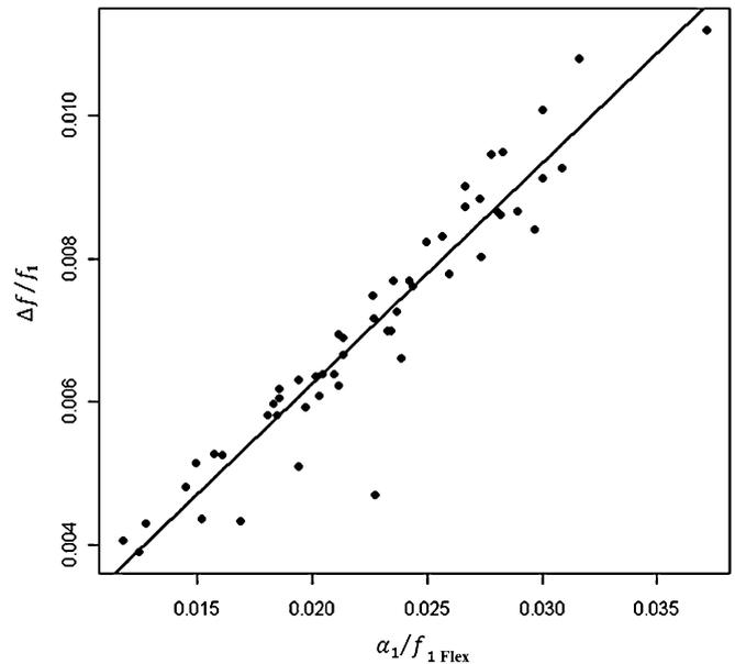
**Fig. 5.** Comparison of results obtained through free vibration  $\alpha_1/f_{1Flex}$  and forced vibration  $\Delta f/f_1 (= Q^{-1})$ , both in bending ( $n = 54$ )
