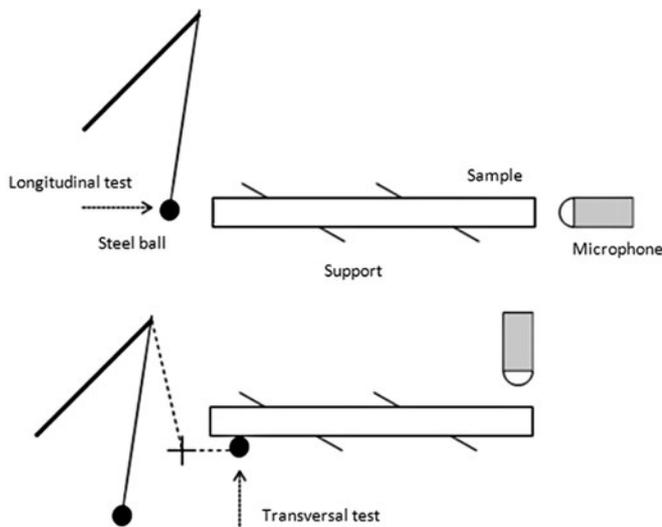
**Fig. 1.** Experimental setup of bending (transversal) and compression (longitudinal) free-vibration device
