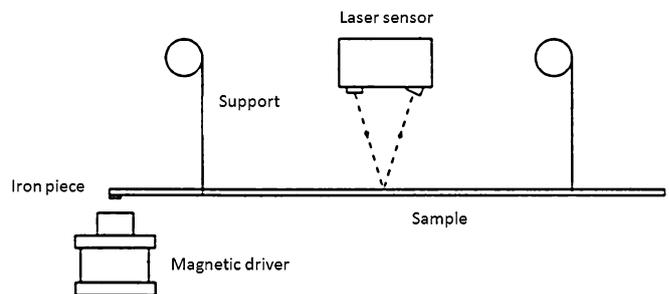
**Fig. 2.** Experimental setup of forced-released bending vibration device
