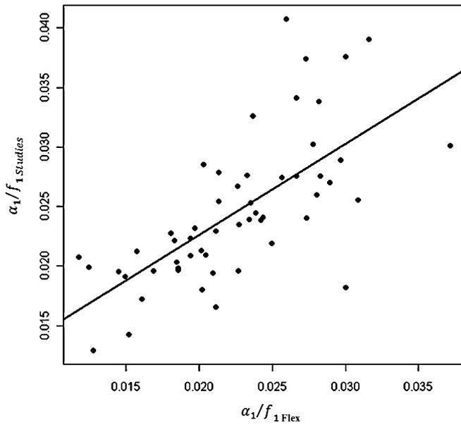
**Fig. 3.** Comparison of results obtained with bending free vibration (temporal damping-to-frequency ratio for the fundamental frequency,  $\alpha_1/f_{1Flex}$ ) compared to previous studies  $\alpha_1/f_{1Studies}$  (Brancheriau et al.<sup>17,18</sup>; Aramaki et al.<sup>19</sup>;  $n = 54$ )
