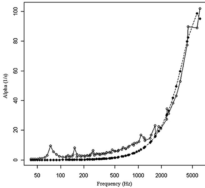
**Fig. 6.** Changes in temporal damping  $\alpha$  according to frequency  $f$  for the Madagascar rosewood specimen (open circles, experimental points; solid circles, adjustment,  $n = 88$ )
