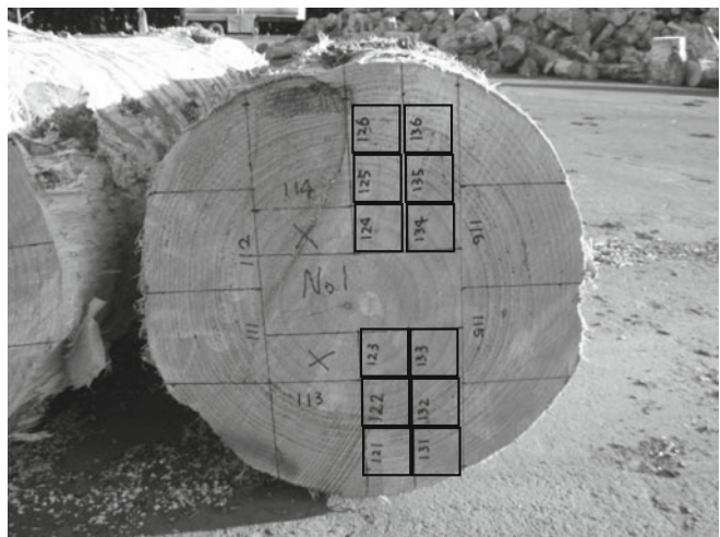
Fig. 2. Locations (enclosed with squares) where timber specimens of radiata pine were extracted. This procedure was different from that for the other species
