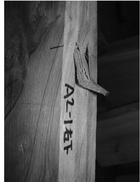
Fig. 9. Shear failure of bamboo nails
