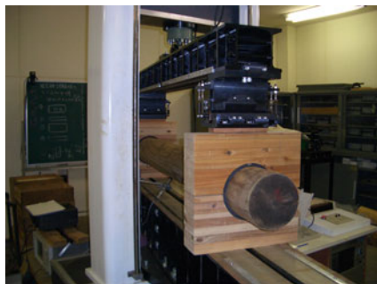
c Tensile and compression testing machine realizing various conditions for actual-size specimens
