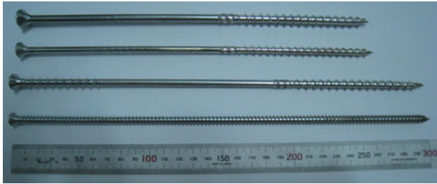
Fig. 1 Self-tapping screws designed for large-scale wood-framing connections. From top to bottom ST10 × 260 with half-threaded shank, ST8 × 260 with half-threaded shank, ST8 × 300 with two threaded sections, ST7.5 × 302 with fully threaded shank
