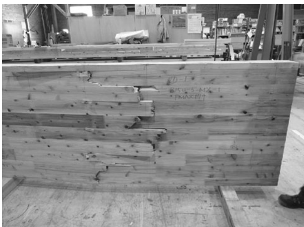
Fig. 12 Typical failure of CLT panel on tension side (type Rd 150 mm 5ply)
