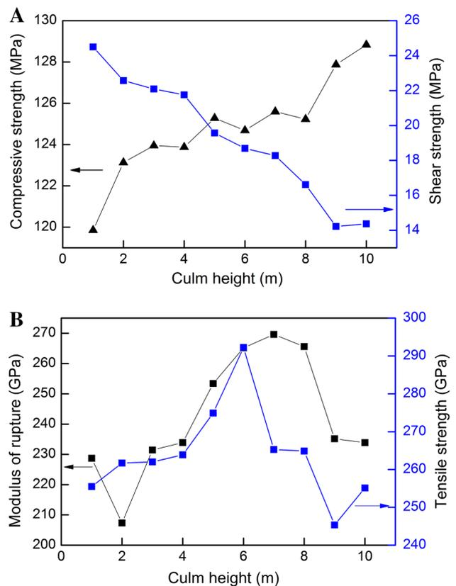
Fig. 2 Effect of culm height on mechanical properties of bamboo plywood
