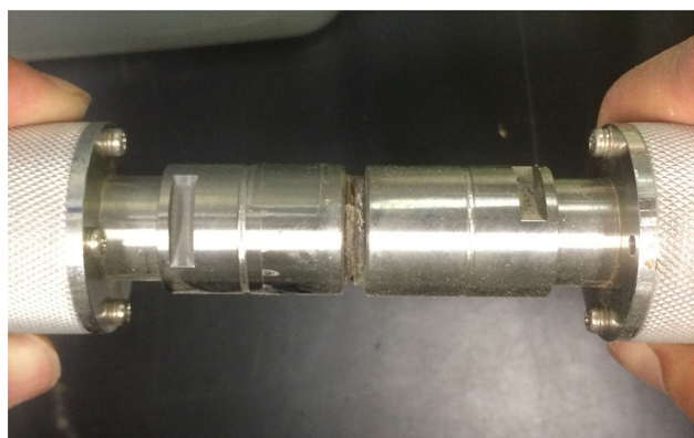
Fig. 3 Measurement of non-attenuated signal. Any attenuating materials were not between the dry couplants
