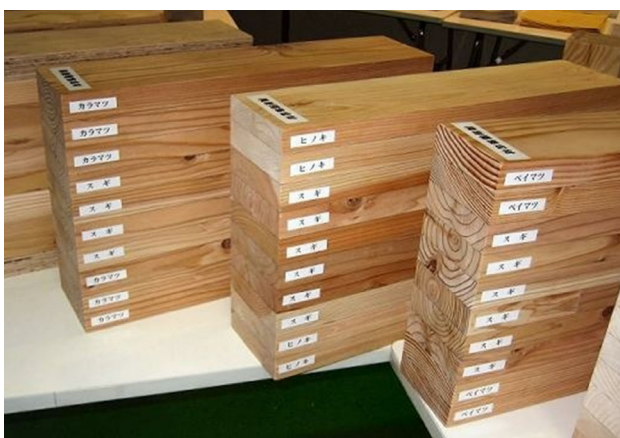
Fig. 2 Sugi composite glulam using karamatsu, hinoki and Douglas fir (from left to right)
