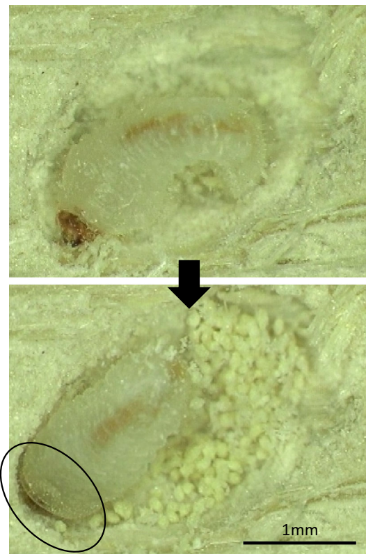
Fig. 8 Part of the bamboo specimen marked with an oval was consumed by Larva II and particles of larval excreta were produced within 4 h
