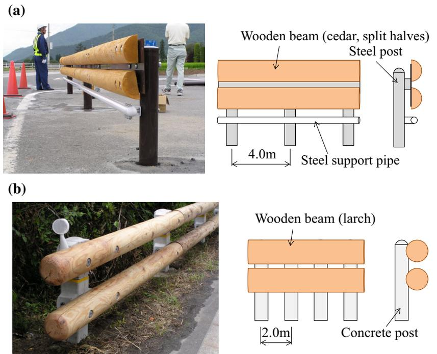
**Fig. 2** Types of steel guardrail. **a** Steel guardrail. **b** Steel guard pipe
