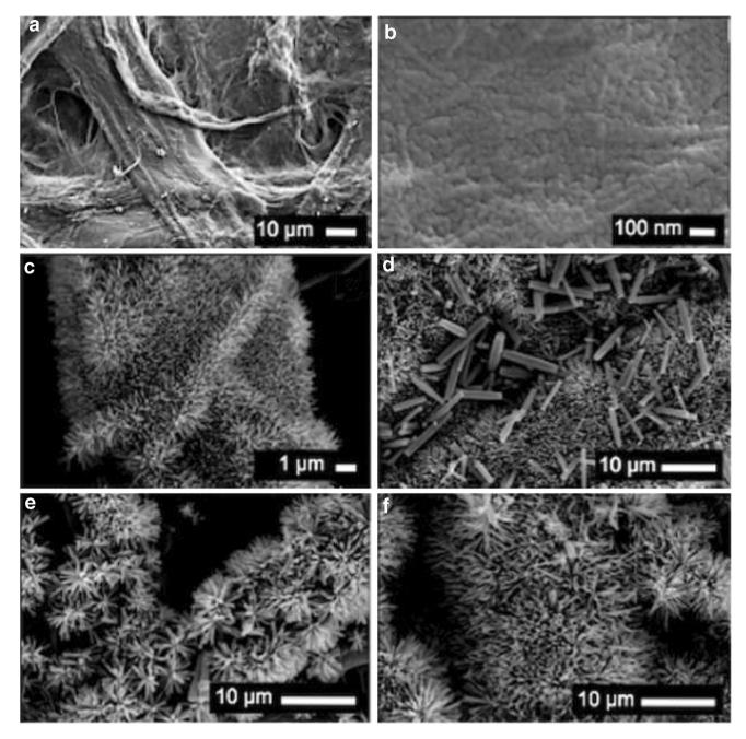
**Fig. 5** SEM micrographs showing **a** untreated handsheet paper; **b** after seeding with ZnO nanoparticles; **c** ZnO nanorods grown on paper at a concentration of 10 mM for 10 h; **d** ZnO nanorods grown
