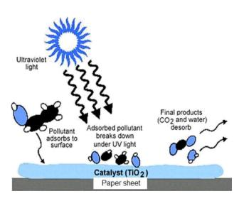
Fig. 4 TiO<sub>2</sub> paper sheet in photocatalysis system [120]
