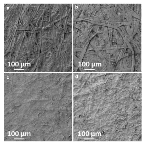
Fig. 3 SEM micrographs of the four paper samples: a standard tracing paper. b laboratory paper sample. c microcrystalline cellulose paper and d Nanocellulose paper [85]
