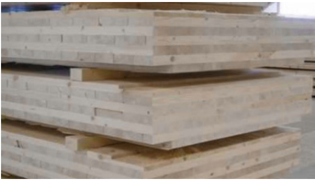
Fig. 1 Layering of cross laminated timber (CLT)
