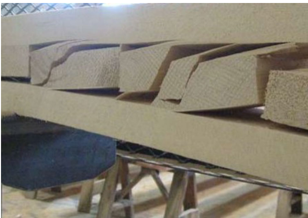
Fig. 2 Rolling shear behaviour in CLT cross layers (shear behaviour in a plane perpendicular to the grain direction)
