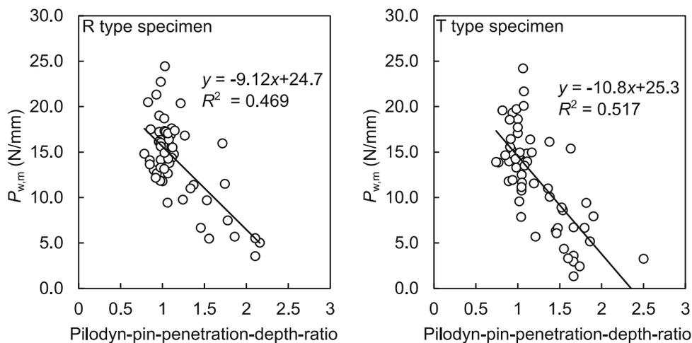
increased, and we estimated  $P_{w, m}$  using mass loss or Pilodyn pin penetration depth. We can estimate the withdrawal strength of nailed joints when the nailed joints were under decay conditions, and rust formed on the penetrated nail, by multiplying the regression lines
