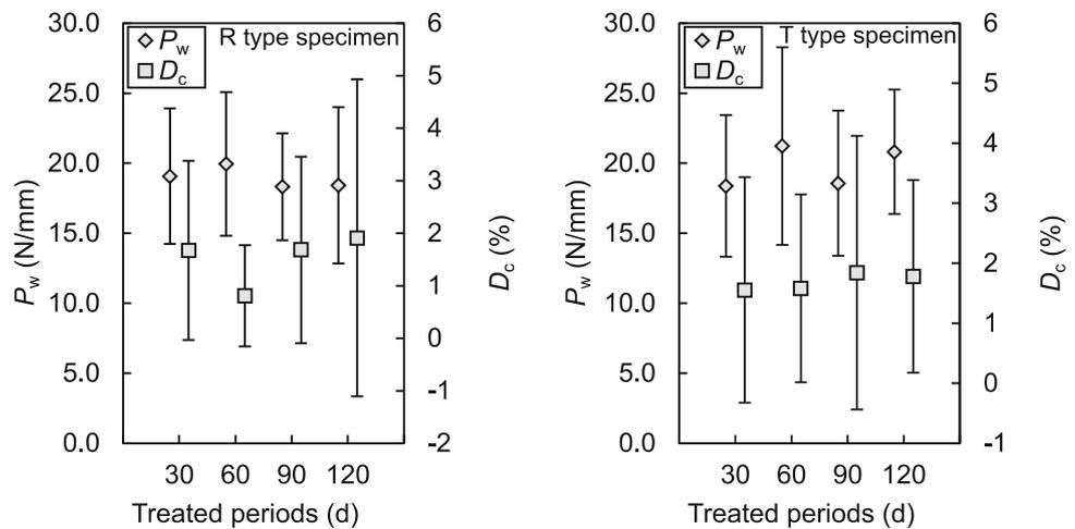
**Effect of nail corrosion on withdrawal strength**
