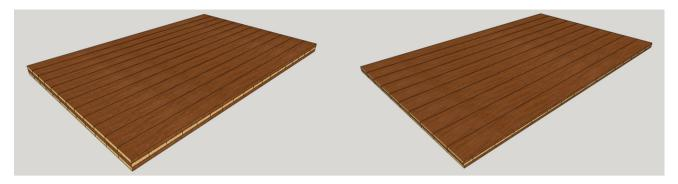
**Fig. 1** CLT plates with 35/35/35 layup and 20/20/20 layup
