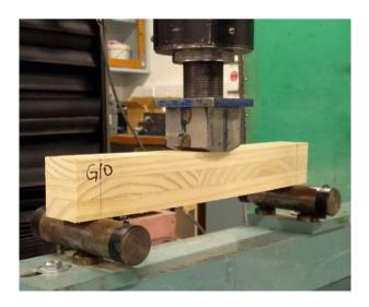
Fig. 2 Short-span bending test setup
