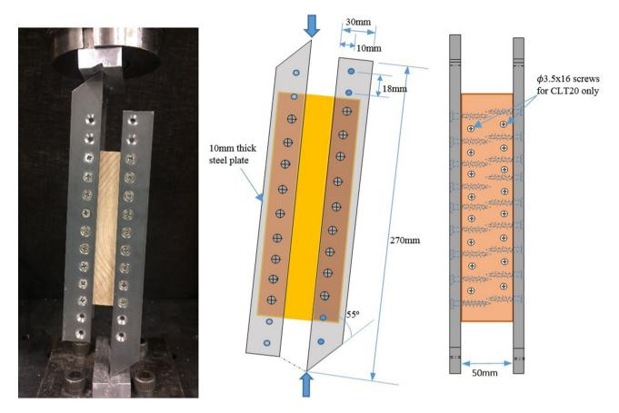
Fig. 3 Modified planar shear test setup
