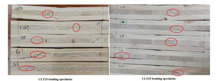
Fig. 4 Typical rolling shear failure modes observed in the bending specimens
