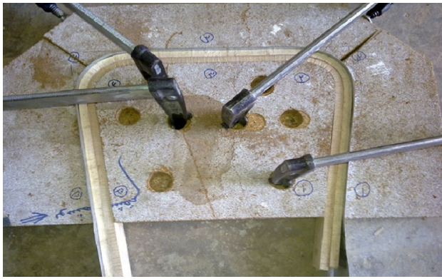
Fig. 2 Fastening clamps attached to the curved parts
