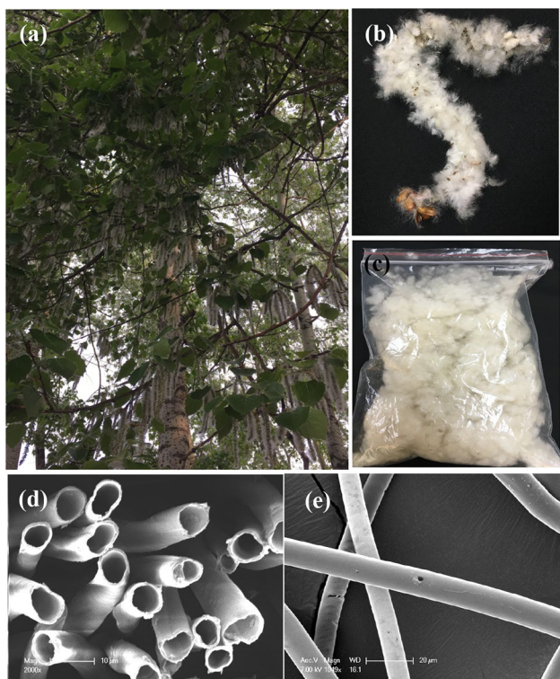
Fig. 1 Photos of poplar catkins that are still on the poplar tree (a) and collected (b), catkin fibers were isolated from the seed by hand (c), SEM images of poplar catkin fiber: d cross section, and e longitudinal
