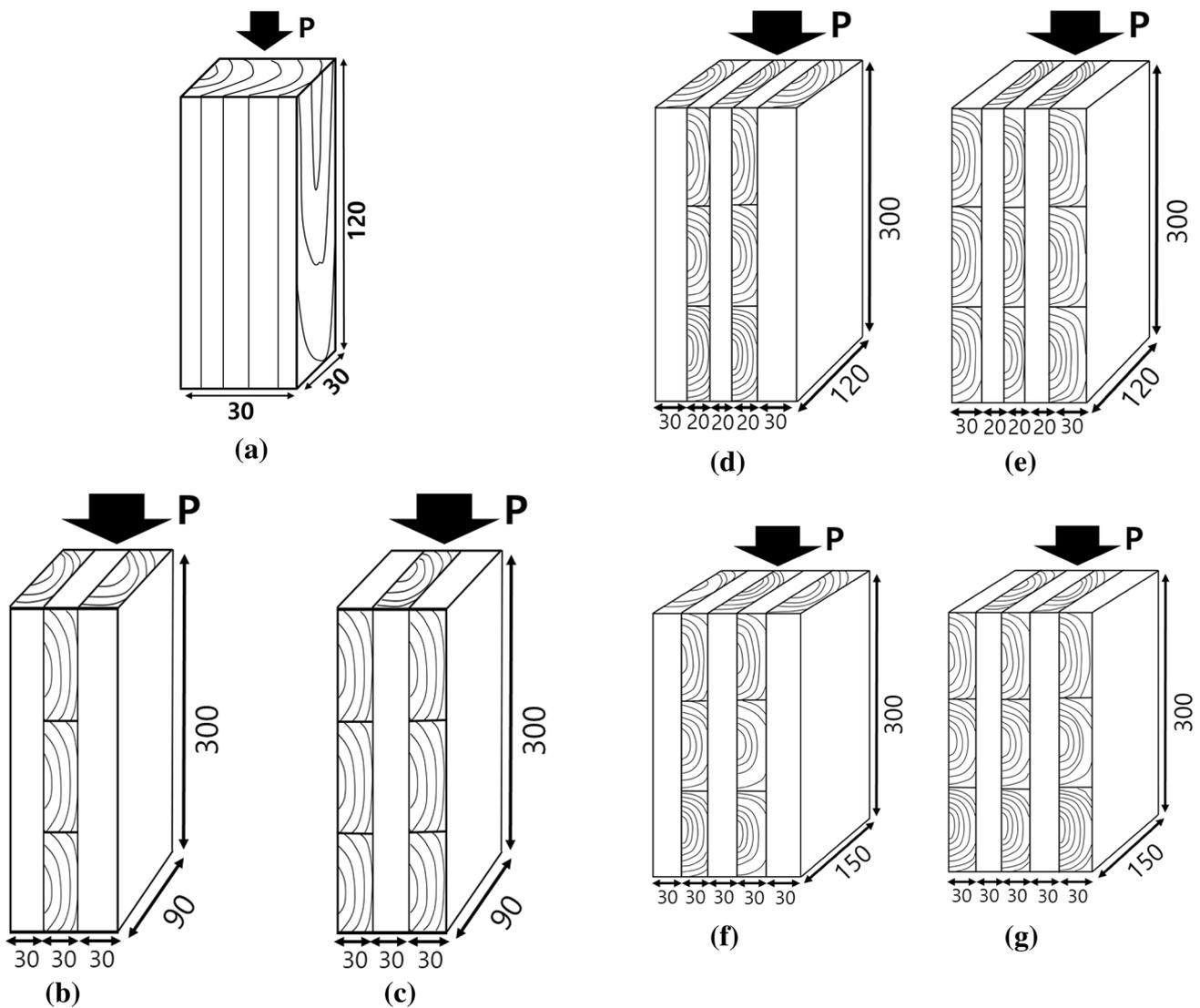
Fig. 3 Specimens for compression test (mm)
