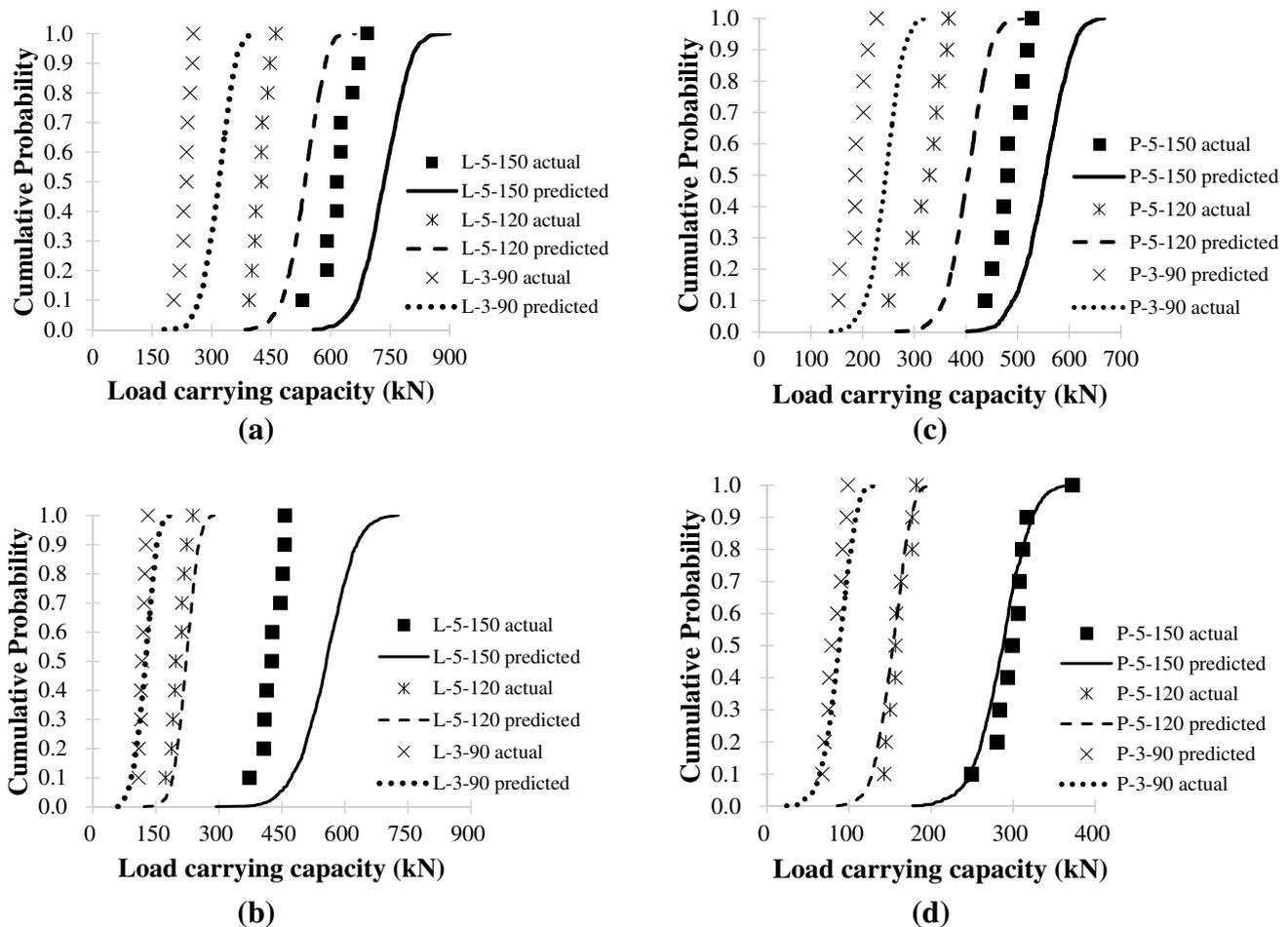
**Fig. 8** Compressive resistance distributions of cross-laminated timber by Method 1
