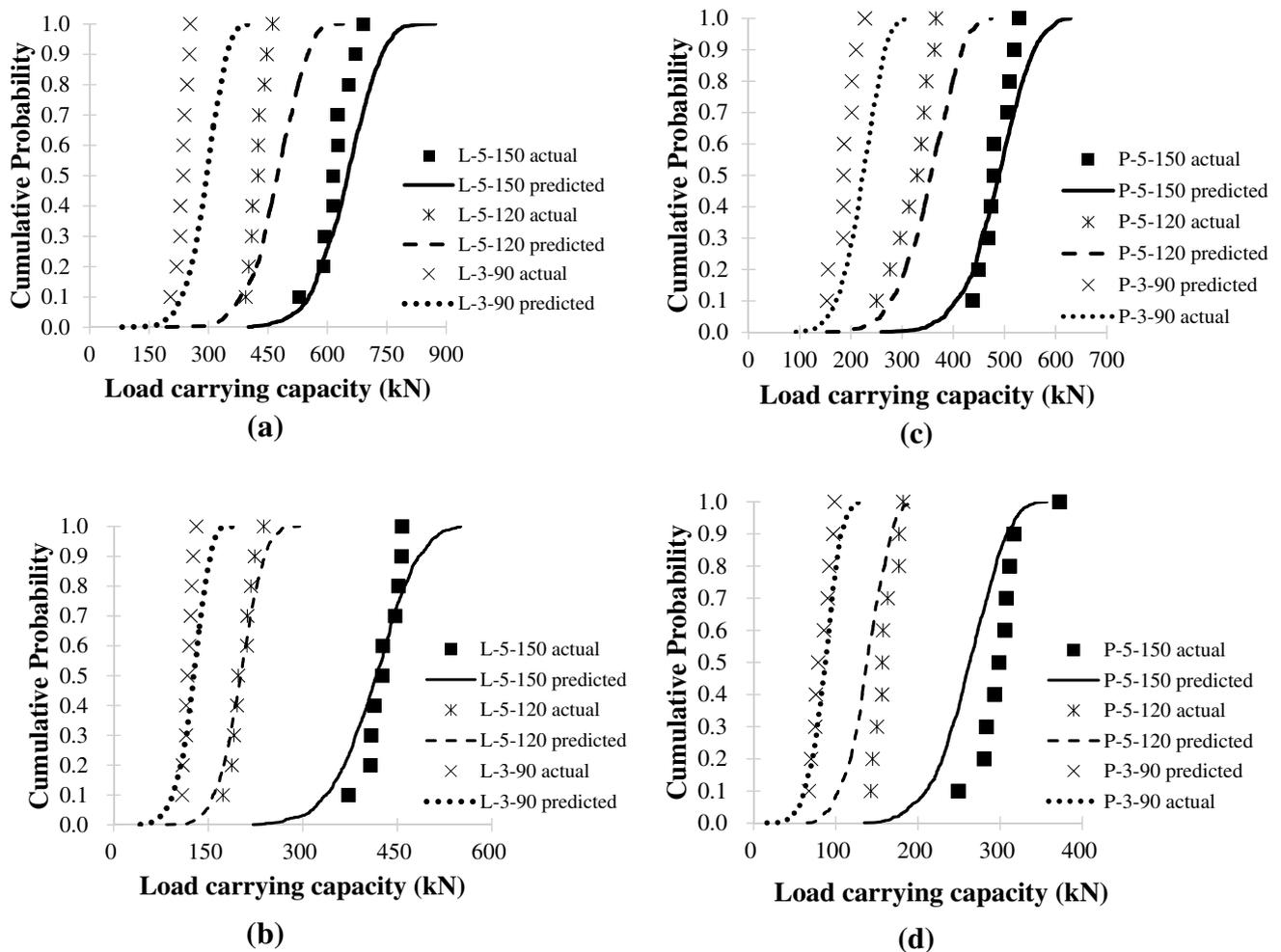
Fig. 10 Compressive resistance distributions of cross-laminated timber by Method 3
