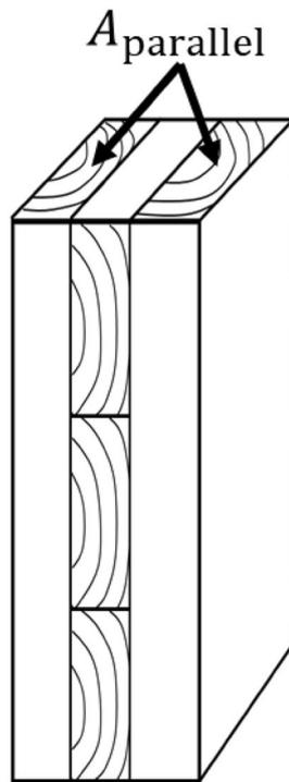
where  $P_{\text{parallel}}$  compressive resistance of CLT,  $\sigma_c$  compression strength of lamina parallel to the loading direction,  $A_{\text{parallel}}$  cross-section area of lamina parallel to the loading direction.
