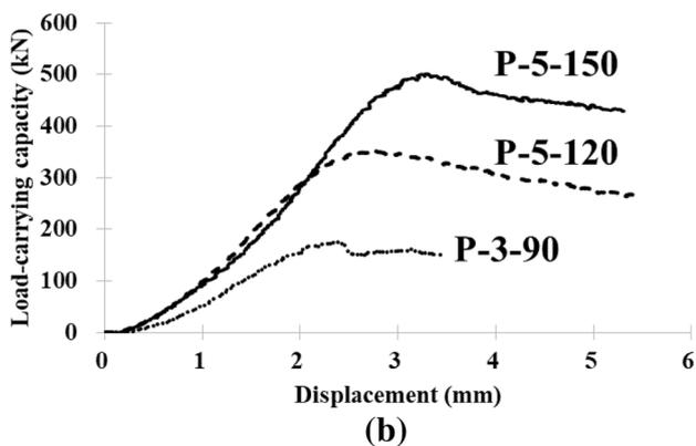
Fig. 6 Load-carrying capacity of CLT in major direction
