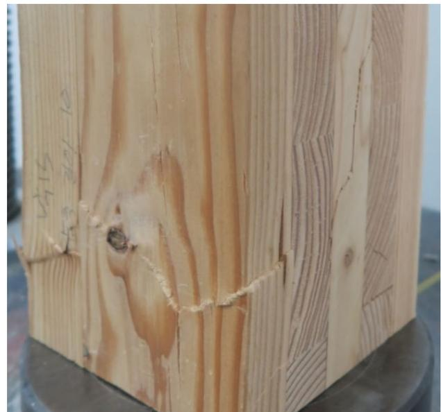
**Fig. 5** Failure mode of cross-laminated timber (crushing)
