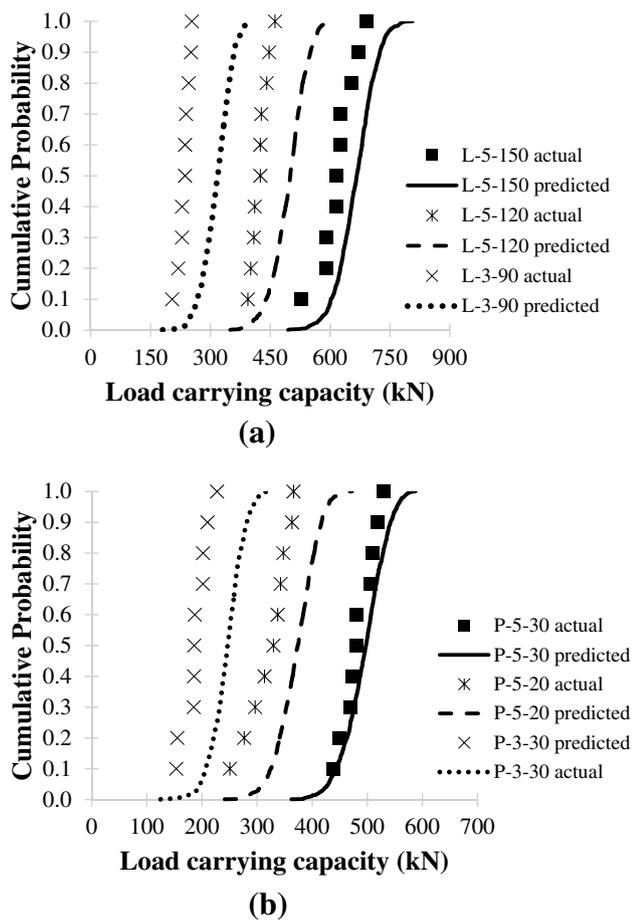
**Fig. 9** Compressive resistance distributions of cross-laminated timber by Method 2
