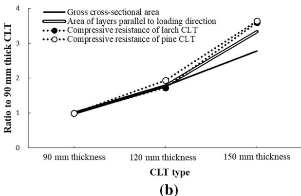
Fig. 7 Gross cross-sectional area, area of layers parallel to the loading direction, and the compressive resistance ratios (90, 120 and 150 mm thick CLT to 90 mm thick CLT)
