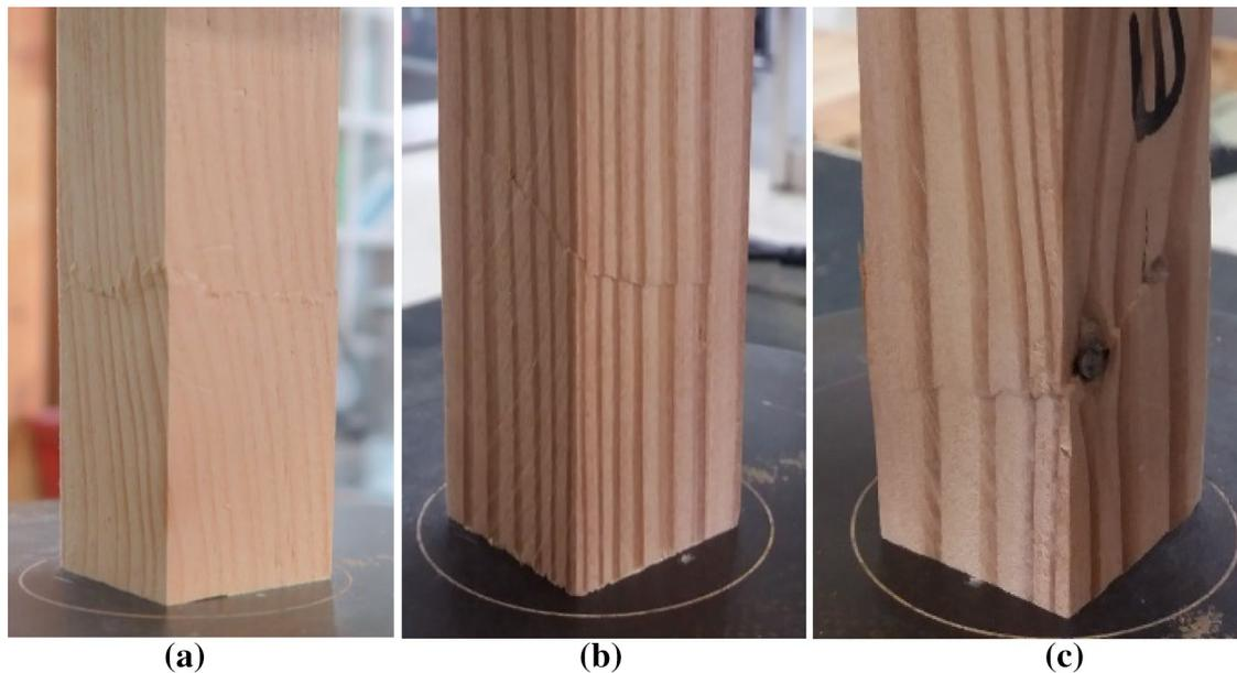
**Fig. 4** Failure modes of lamina specimens
