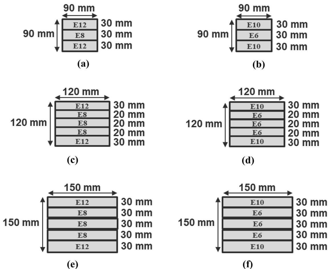
**Fig. 2** Lamina grades and lay-up of CLT specimens
