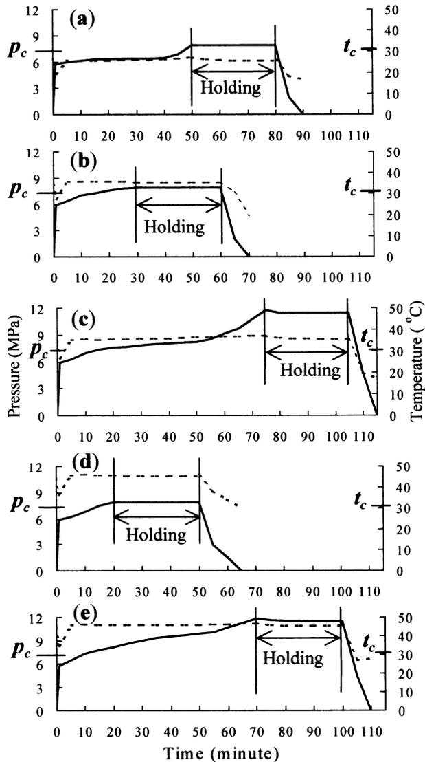
**Fig. 4a–e.** Pressure and temperature changes during supercritical fluid impregnation into wood-based composites at 25°C/7.85 MPa (a), 35°C/7.85 MPa (b), 35°C/11.77 MPa (c), 45°C/7.85 MPa (d), and 45°C/11.77 MPa (e) with a holding time of 30 min. *Solid lines*, pressure level; *dashed lines*, temperature level. CO<sub>2</sub> critical pressure (7.40 MPa) and critical temperature (30.84°C) are indicated by  $p_c$  and  $t_c$ , respectively.
