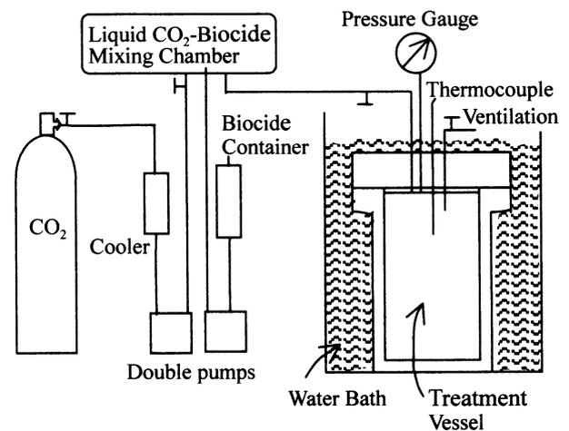
Fig. 1. Apparatus used for supercritical-carbon dioxide (SC-CO<sub>2</sub>) treatment
