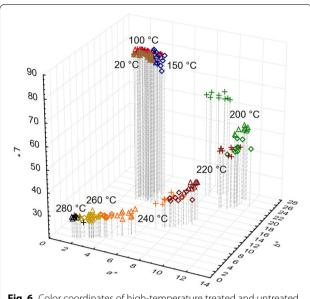
Fig. 6 Color coordinates of high-temperature treated and untreated fir wood. Each color represents a specific temperature of treatment. Signs +,  $\triangle$  and  $\diamondsuit$  stand for 1-h, 3-h and 5-h treatment, respectively
