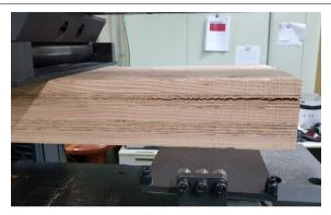
a Rolling shear failure
