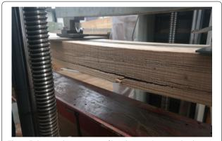
**Fig. 5** Failure modes specimen of bending test (span-to-depth ratio was 25:1)
