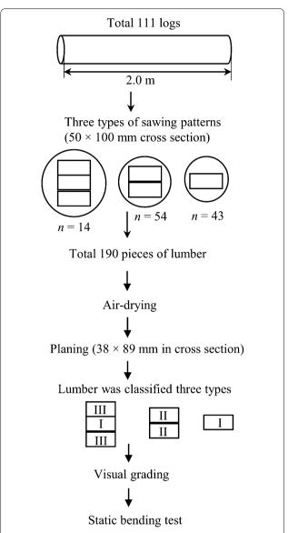
**Fig. 1** Illustration of the experimental procedure. *n* number of logs. Among the large diameter logs, four lumber (one lumber was type I, and three pieces of lumber were type III) were obtained from one log. Totally, 194 pieces of lumber were obtained from 111 logs. However, we failed to collect the data of bending tests for four pieces of lumber. Thus, totally 190 pieces lumber data were used
