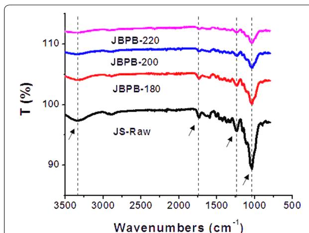
**Fig. 3** Fourier transform infrared spectra of jute stick particles and manufactured jute stick binderless particleboard (JBPB) as a function of press temperatures
