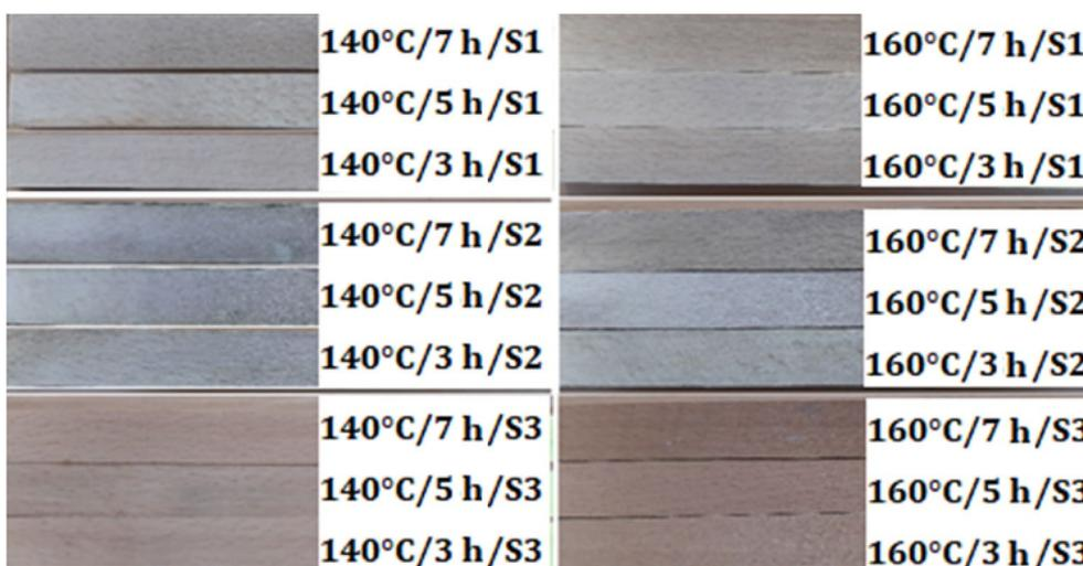
**Fig. 7** Heat-treated beech samples after bleaching treatment
