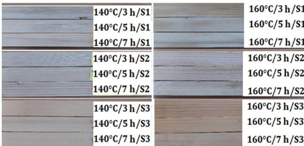
**Fig. 5** Heat-treated fir samples after bleaching treatment
