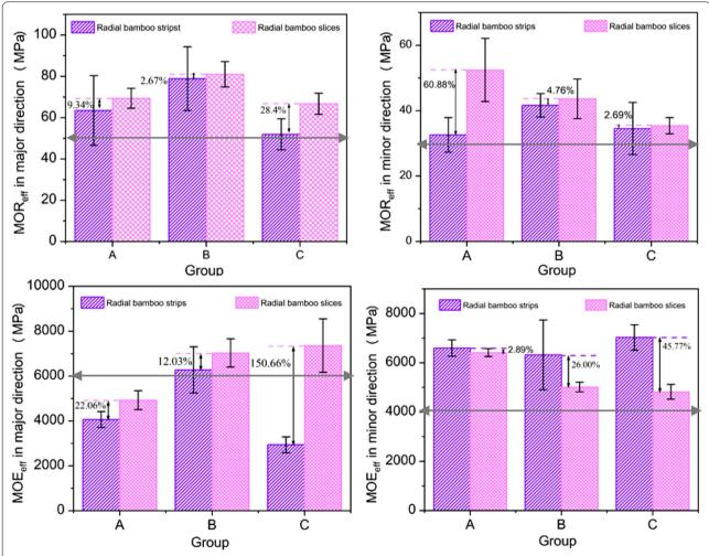
Fig. 7 MOReff and MOEeff of different layups in major and minor direction. Note " ↔ " means the baseline of standard GB/T17656-2018 [20]. Error bar indicates the C.V. of MOReff and MOEeff
