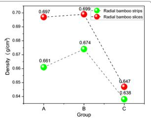
**Fig. 5** Density of different layups. Note group **A** consists of poplar veneer and bamboo mat as surface layer. Group **B** consists of two bamboo mats as surface layer. Group **C** consists of two poplar veneers as surface layer
