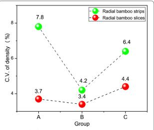
**Fig. 6** C.V. of different layups. Note group **A** consists of poplar veneer and bamboo mat as surface layer. Group **B** consists of two bamboo mats as surface layer. Group **C** consists of two poplar veneers as surface layer
