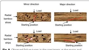
**Fig. 8** Observed failure types in the specimens at the major and minor strength directions during bending testing
