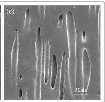
Fig. 13 Gas-assisted laser cut wood surface optimization. a Traditional laser machining. b Gas-assisted laser processing. c Micromorphology of kerf surface
