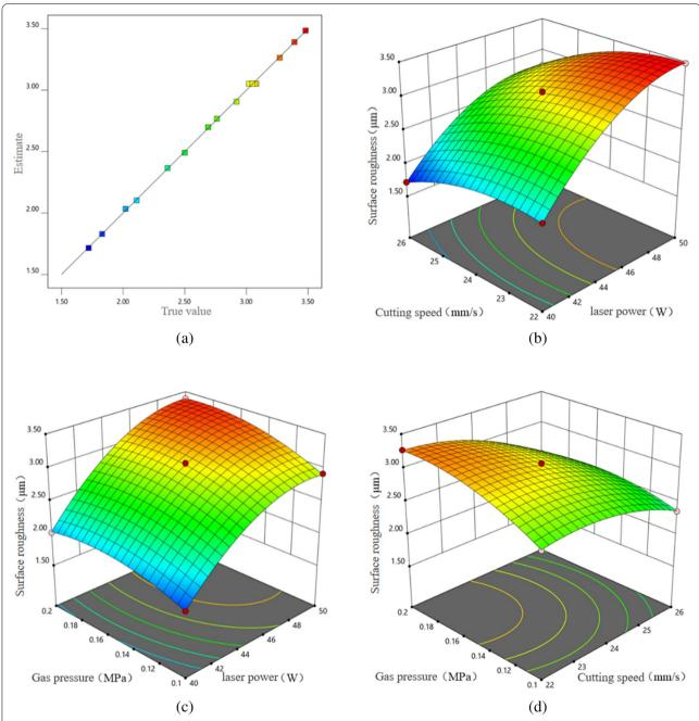
**Fig.12** Response surface diagram of surface roughness of inert gas-assisted laser cutting wood. **a** Comparison between predicted and actual. **b** Interaction of laser power and cutting speed. **c** Interaction of laser power and gas pressure. **d** Interaction of cutting speed and gas pressure
