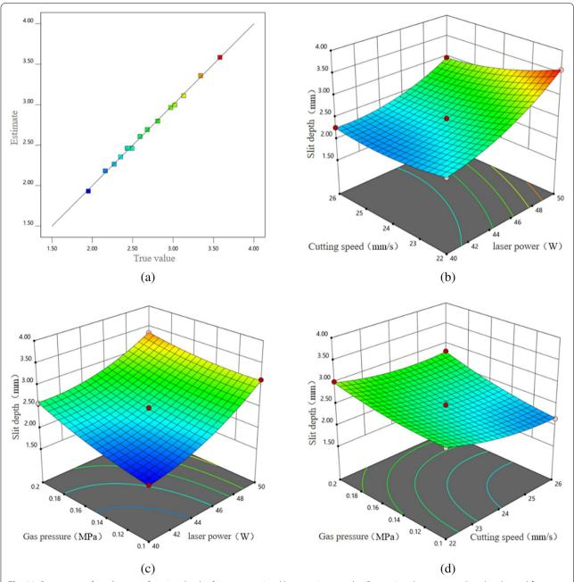
Fig. 11 Response surface diagram of cutting depth of inert gas-assisted laser cutting wood. a Comparison between predicted and actual. b Interaction of laser power and cutting speed. c Interaction of laser power and gas pressure. d Interaction of cutting speed and gas pressure
