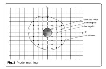
For the explicit difference scheme, the discrete solution of unsteady heat transfer process needs to be considered in the stability condition. The above explicit difference formula displays that the temperature of the time node n+1 on the space node I is affected by the adjacent points on the left and right sides, and the stability limit condition (Fourier grid number limit) needs to be satisfied, otherwise there would be unreasonable oscillatory solutions[16].
