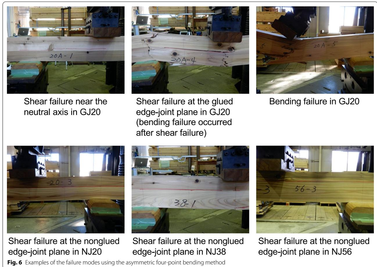
**Fig. 6** Examples of the failure modes using the asymmetric four-point bending method
