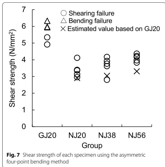
Fig. 7 Shear strength of each specimen using the asymmetric four-point bending method
