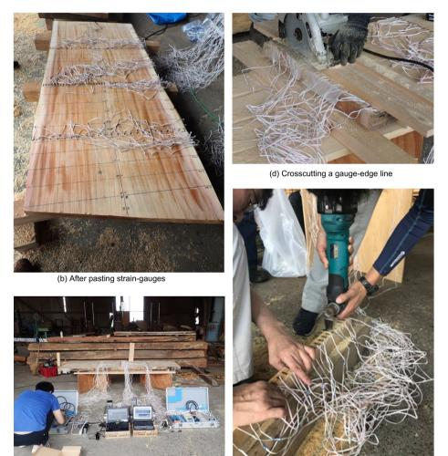
(c) Strain-gauges connected to data loggers
