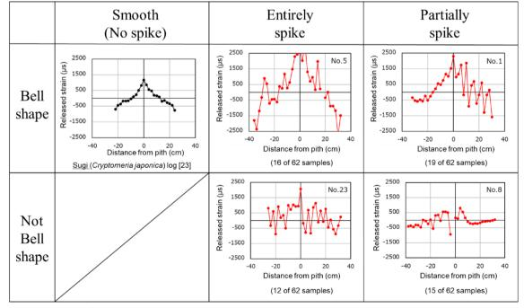
Fig. 5 Typical distribution of released stain in an upright tree of Japanese cedar (*Cryptomeria japonica* D. Don) [24]) and four representative types of distribution pattern of keyaki wood measured in this study (sample Nos. 1, 5, 8, and 23). Plus and minus signs of the horizontal axis were occasionally given depending on the experimental situation
