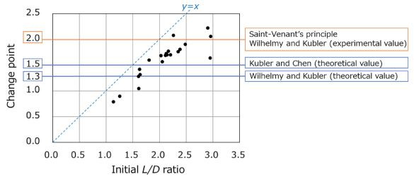
Fig. 10 Relationship between the change point (y) and the value of initial L/D ratio (x) and the comparison with the thresholds of previous researches [36–39]. Initial L/D was calculated as half of the plank length divided by log diameter
