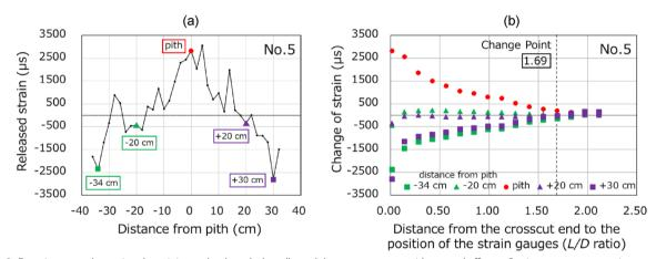
Fig. 9 Experiment to determine the minimum log length that allowed the measurement without end effect. **a** Strain measurement points on the pith, the outermost part of xylem, and the midpoints between them whose strain values were followed by 10-cm crosscutting (e.g., sample No. 5). **b** Change of strain values at the five strain measurement points. Change point: *L/D* ratio of crosscut position where the strain values began to change obviously
