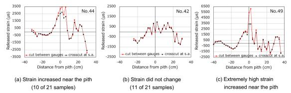
Fig. 8 Changes in strain due to cutting between the strain gauges. (It is noted that the maximum values of the vertical axis are not the same)
