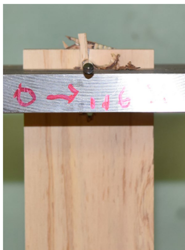
Fig. 4 End shear failure (ESF). The parameters were as follows: panel type, PW-s; d , 5.2 mm; ph , 0; dowel position, A
