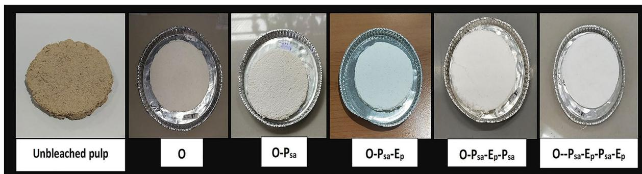
**Fig. 6** Transformation of SPF unbleached pulps into pure cellulose during five-stage TCF bleaching at 23% AA dosage (O: oxygen; P<sub>sa</sub>: peroxymonosulfuric acid; E<sub>p</sub>: alkaline extraction with hydrogen peroxide)
