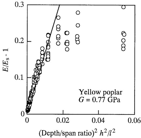
**Fig. 2.** Value of  $(E/E_s - 1)$  calculated by substituting the shear modulus obtained from the vibration tests into Timoshenko's bending theory corresponding to the squares of depth/span ratio
