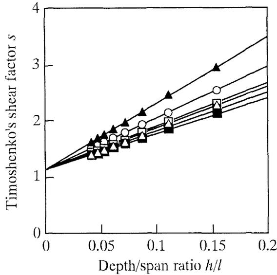
**Fig. 4.** Dependence of Timoshenko's shear factor on the depth/span ratio obtained from the FEM calculations. *Open circles*, spruce; *open squares*, Sugi; *open triangles*, Douglas fir; *solid circles*, red melanti; *solid squares*, buna; *solid triangles*, balsa
