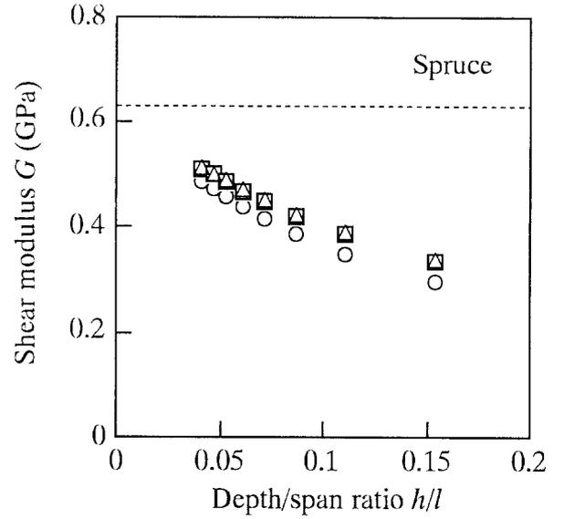
**Fig. 3.** Shear modulus corresponding to the depth/span ratio obtained from the finite element method (FEM) calculations when the grid point for measuring the deflection was varied. *Circles*, measured at the loading point; *squares*, measured at the middle of the depth; *triangles*, measured at the opposite side of the loading point; *broken line*, shear modulus given as a material parameter ( $G = 0.63$  GPa for spruce)
