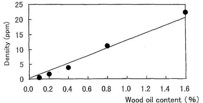
Fig. 8. Calibration curve for the density variation of  $\alpha$ -pinene by gas chromatography corresponding to the concentration of wood oil contained in respective test samples of *C. obtusa*
