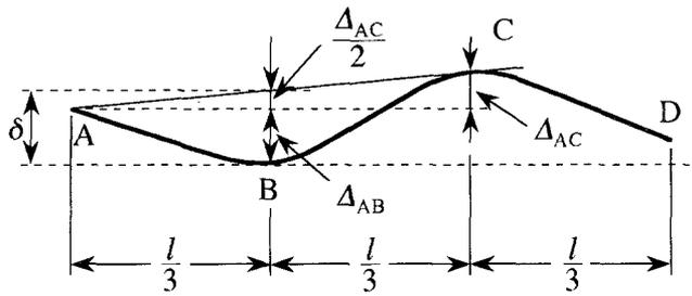
Fig. 2. Definition of vertical displacements in asymmetric four-point bending
