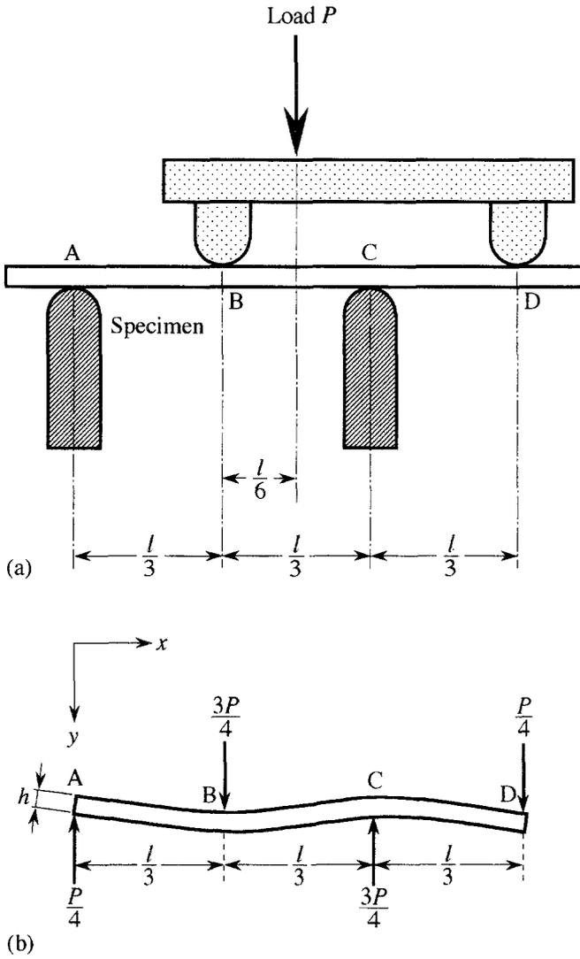
**Fig. 1.** Asymmetric four-point bending test and the beam subjected to the lateral forces
