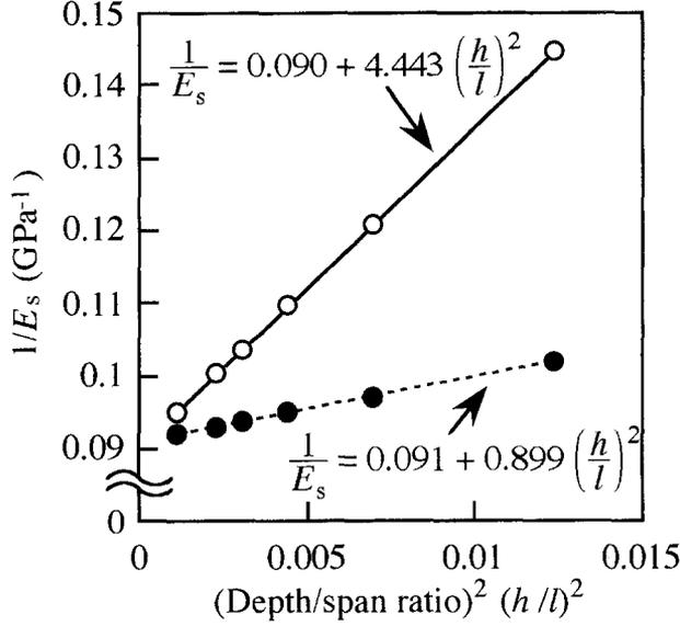
**Fig. 4.** Value of  $1/E_s$  corresponding to the  $(\text{depth}/\text{span ratio})^2$  obtained by the finite element method. *Open and filled circles* are obtained from the simulations of asymmetric four-point and three-point bending tests, respectively; and *dashed lines* are obtained from the regressions of the  $1/E_s-(h/l)^2$  relations of asymmetric and three-point bending simulations, respectively, into linear relations
