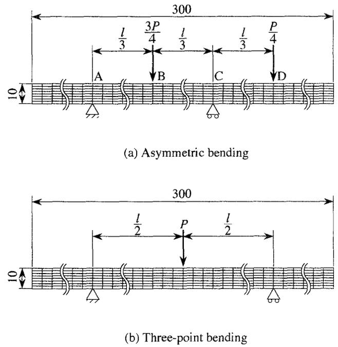
Fig. 3. Finite element meshes used in the numerical calculations. Meshes are uniformly divided to the dimensions of  $5.0 \times 1.25$  mm
