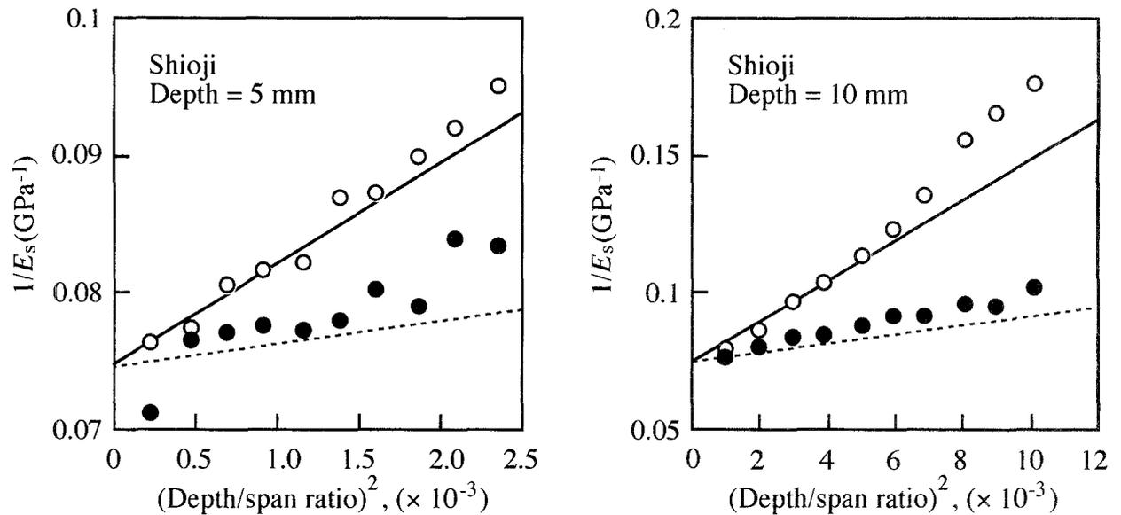
**Fig. 5.** Examples of the inverse values of apparent Young's moduli corresponding to the squares of depth/span ratios. Blank and solid circles are obtained from the asymmetric four-point and three-point bending tests, respectively. *Solid and dashed lines* were obtained by
