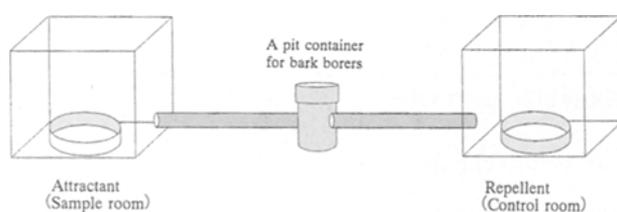
Fig. 1. Olfactometer used for bioassays
