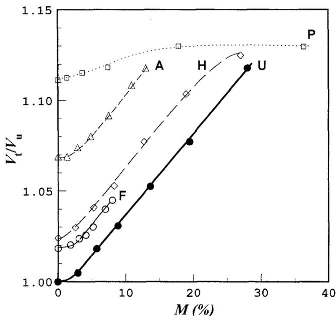
**Fig. 2.** Volumetric swelling ( $V_t/V_u$ ) of untreated and chemically treated wood specimens plotted against the equilibrium moisture content ( $M$ ). The volume ratio,  $V_t/V_u$ , is based on the volume of specimens dried completely in their untreated state
