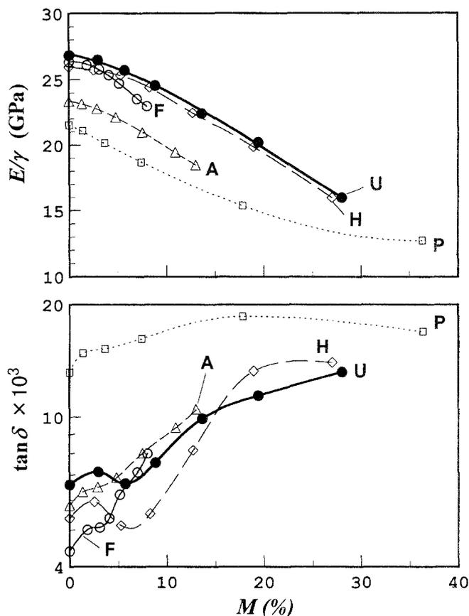
**Fig. 4.** Moisture dependencies of  $E/\gamma$  and  $\tan \delta$  for the untreated and chemically treated wood specimens
