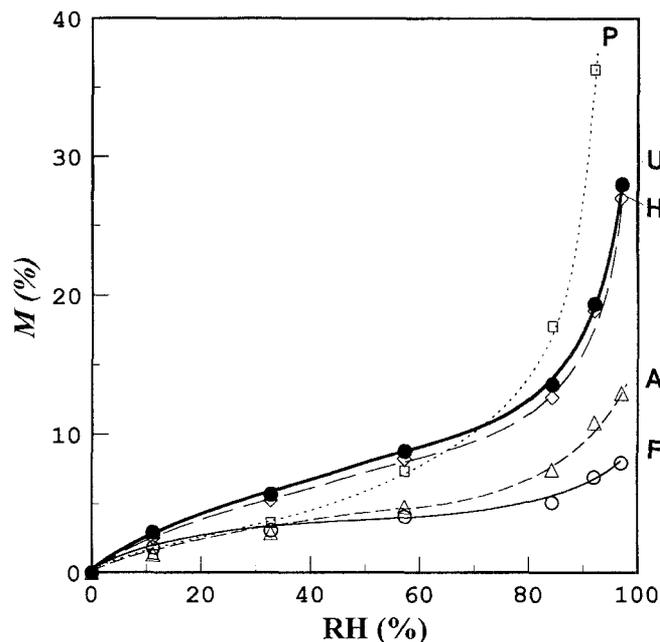
**Fig. 1.** Water sorption isotherms of untreated and chemically treated wood specimens at 25°C. Filled circles, untreated (U); open circles, formalization (F); triangles, acetylation (A); squares, polyethylene glycol impregnation (P); diamonds, hematoxylin impregnation (H);  $M$ , equilibrium moisture content; RH, relative humidity
