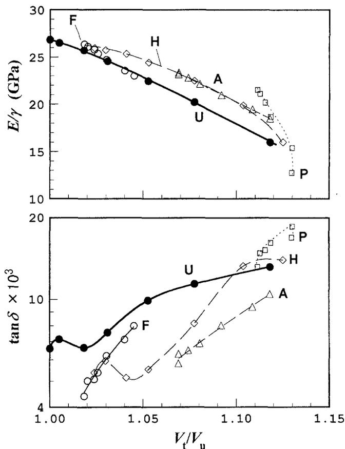
Fig. 5.  $E/\gamma$  and  $\tan\delta$  values of the untreated and chemically treated wood specimens plotted against the volume ratio,  $V_t/V_u$ .
