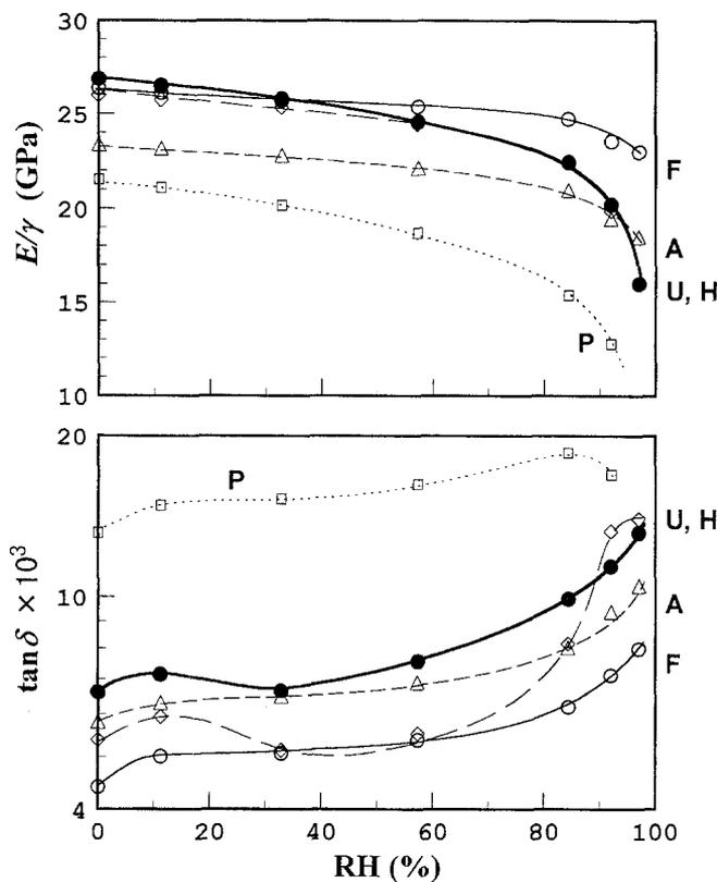
**Fig. 3.** Effects of relative humidity (RH) on the specific dynamic Young's modulus ( $E/\gamma$ ) and loss tangent ( $\tan \delta$ ) of the untreated and chemically treated wood specimens
