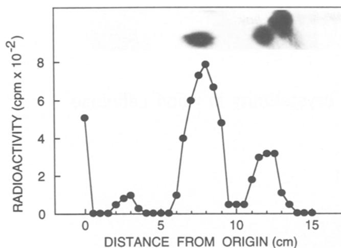
**Fig. 2.** Paper chromatography of the products generated by Smith degradation of [<sup>14</sup>C]sucrose-derived  $\beta$ -glucan. The paper was excised every 5 mm, and its radioactivity was counted with Aquasol. The radioactivity is shown by circles; and the chromatogram of glucose, erythritol, and glycerol is shown at the top of the figure. The sugars were stained with alkaline silver nitrate
