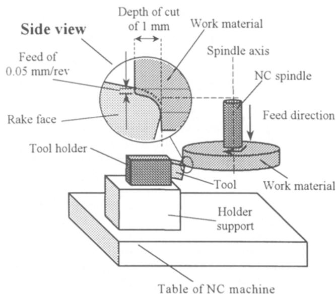
**Fig. 1.** Experimental setup. NC, numerically controlled
