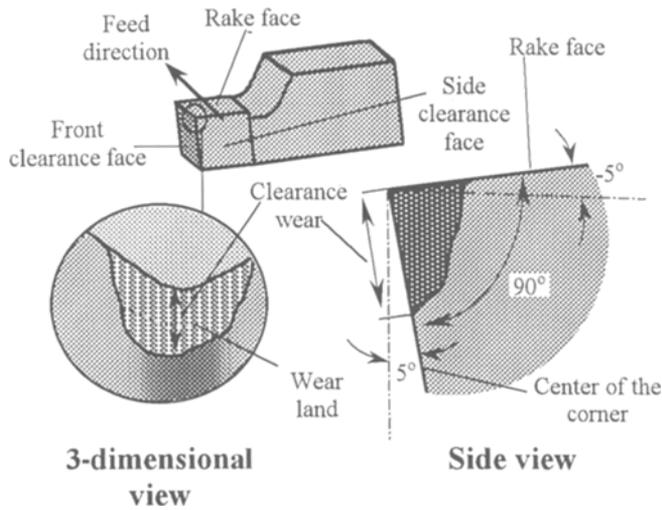
Fig. 2. Clearance wear measurement
