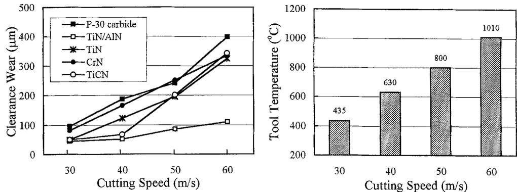
more, the hardness decreased at 800°C. The hardness of the TiCN coating was reported to be about 1100HV at 800°C.<sup>6</sup> These data suggest that the wear rate and clearance wear of the TiCN-coated carbide tool were accelerated by oxidation of its coating film and the decreased hardness due to the high temperature.
