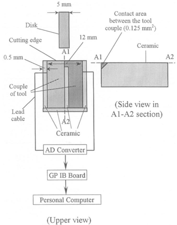
Fig. 3. Thermal electromotive force (EMF) measurement. AD, Analog to digital; GP IB, General purpose interface bus
