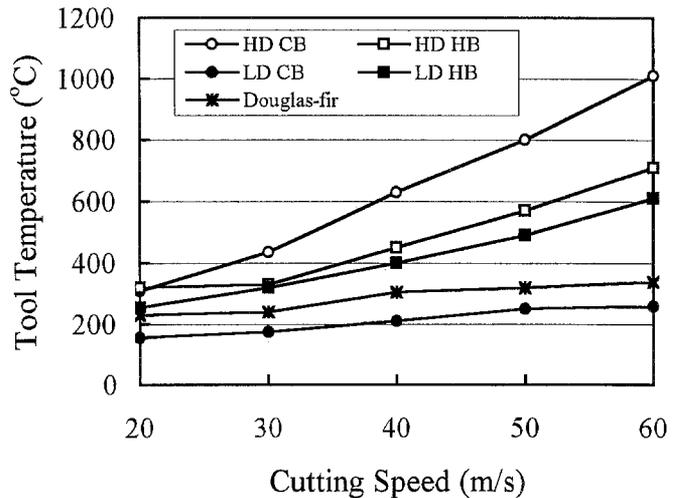
Fig. 4. Cutting tool temperatures as a function of the cutting speeds and work materials. HDCB, high-density wood-chip/cement board; HDHB, high-density hardboard; LDCB, low-density wood-chip/cement board; LDHB, low-density hardboard. Conditions: depth of cut (D) 0.05 mm; width of cut (W) 5 mm; cutting period 3 s. tools were K10 and cermet
