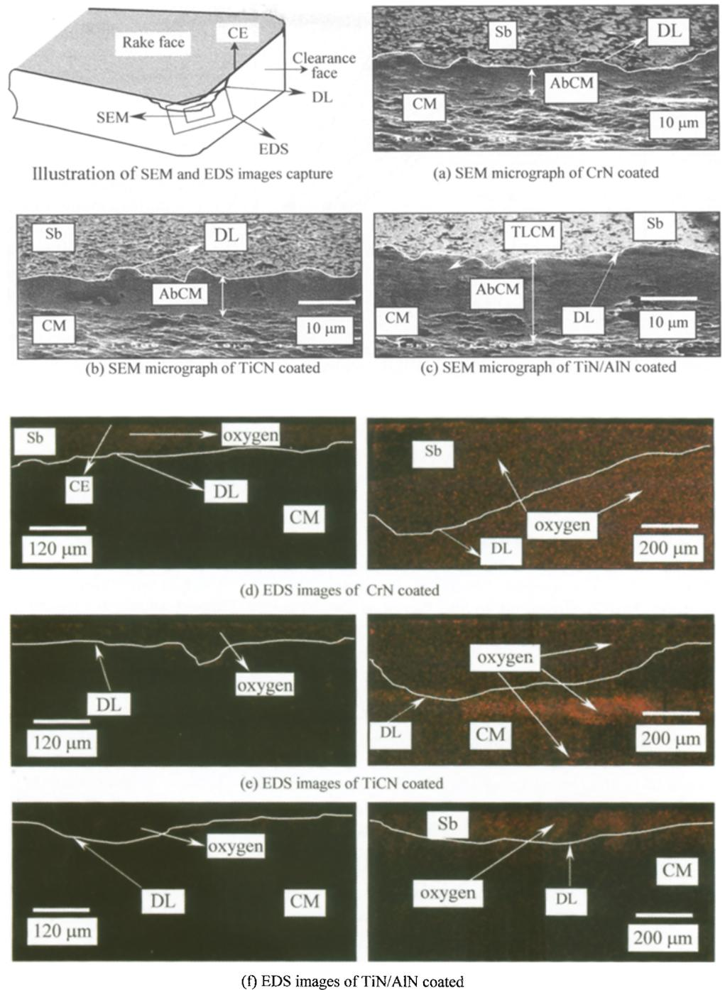
and 60 m/s cutting speeds, respectively (Fig. 6, right) are thought to be responsible for the damage to the substrate due to a severe loss of hardness. The hardness of P grade carbide (10% Co/84% WC) was reported to be about 600 HV at 800°C and 500 HV at 900°C.<sup>7</sup>
